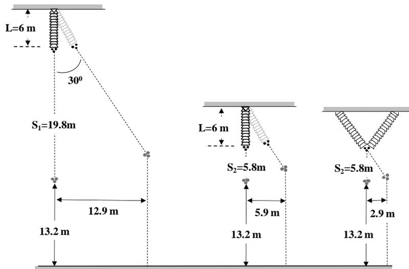
Figure 4 Sag's effect on tower height and ROW width
