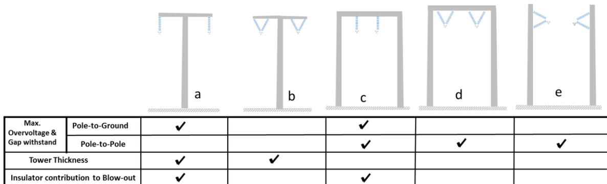
Figure 5 Basic tower configuration options and configuration-related factors effecting poles spacing
