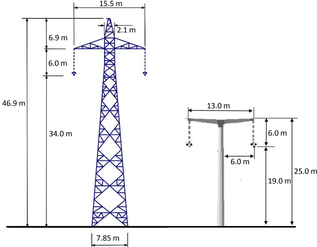
Figure 6 Comparison of HVDC Tower Options with equal mid-span ground clearance and thermal loading of 3800 MW at 500 kV [9],[13]
