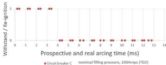
Figure 6: Circuit-breaker C arcing window.
