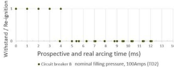
Figure 5: Circuit-breaker B arcing window.
