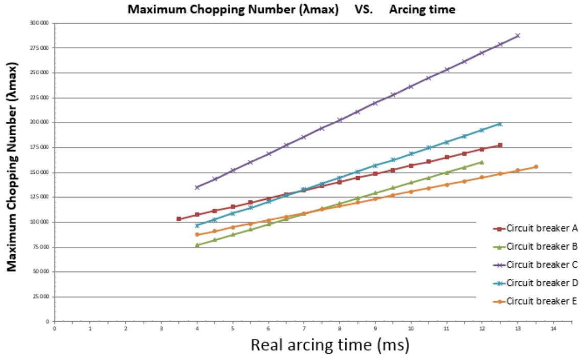
**Figure 10: Maximum chopping number versus arcing time for the five circuit-breakers considered.**
