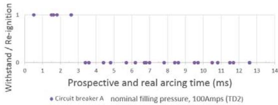
Figure 4: Circuit-breaker A arcing window.
