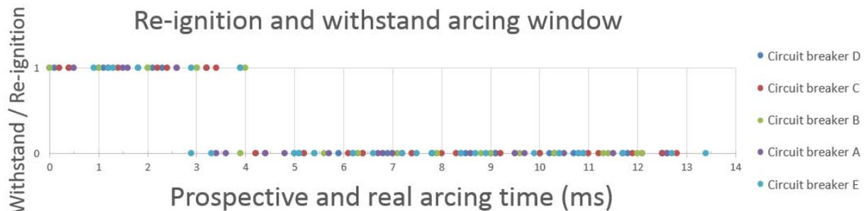
Figure 9: Comparisons of all five circuit-breaker's arcing window
