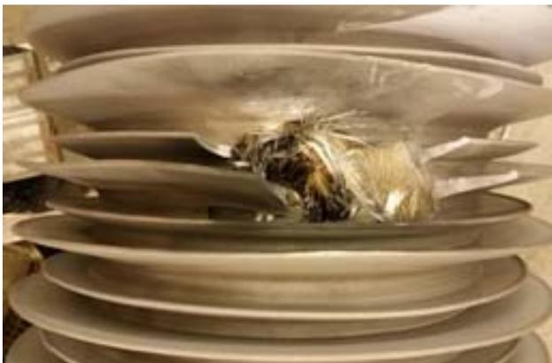
**Figure 2: Perforation of composite circuit-breaker.** **Figure 3: Perforation of the composite insulator.**
