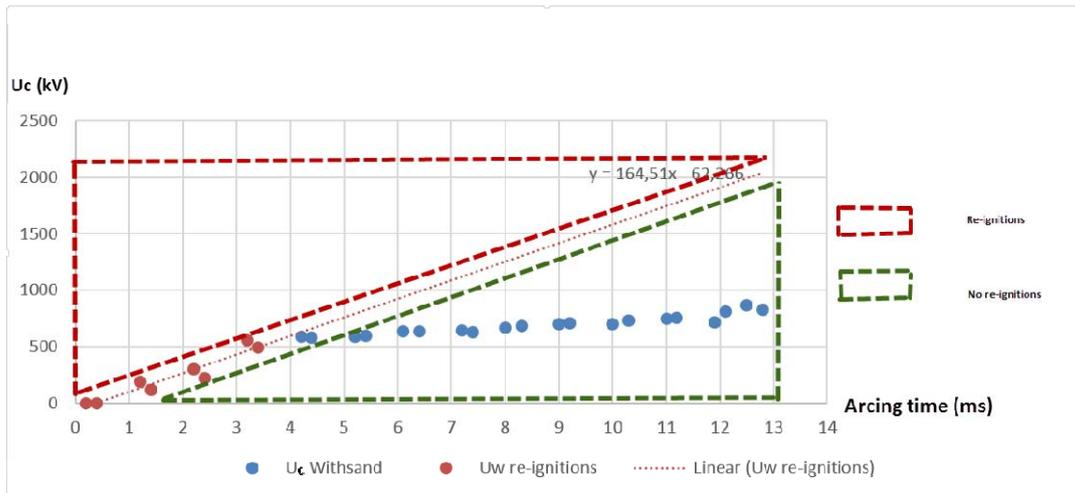
**Figure 11: Dielectric strength versus time for circuit-breaker C.**
