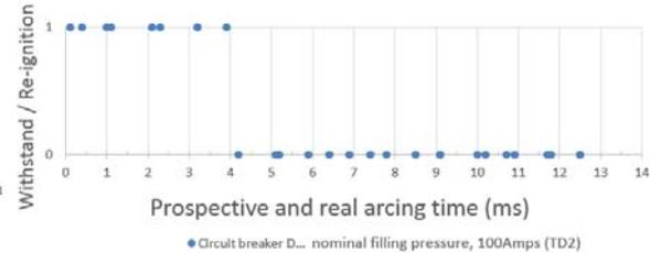
Figure 7: Circuit-breaker D arcing window.
