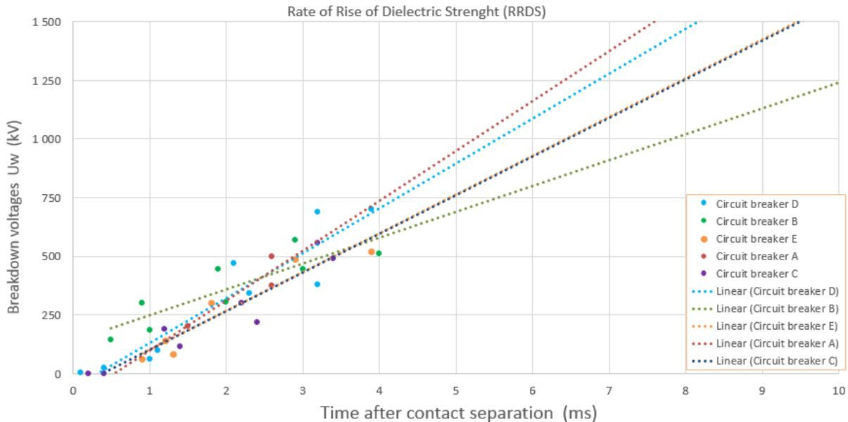
**Figure 12: Estimate dielectric strength versus time for the five circuit-breakers.**
