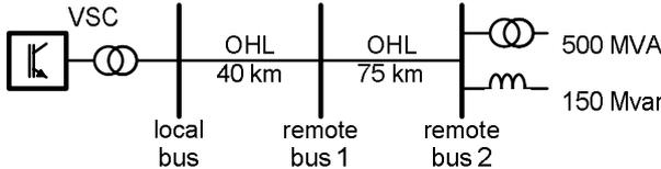
bus. At this second bus a 150 Mvar shunt reactor was additionally put into operation. Finally an unloaded 500MVA transformer was energized at the second remote bus. The test sequence was performed with the primary voltage control set to a 400 kV
