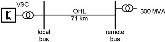
interconnecting the HVDC bus bar via a 71 km long 400 kV transmission line with a remote bus. To this bus an unloaded 300 MVA transformer was connected. The test was performed with the primary voltage control set to a 360 kV target value with a
