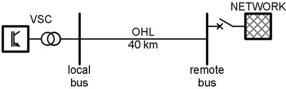
After re-synchronization the HVDC was operated in U/f-Mode for approximately an additional 40 minutes. During this time the power dispatch in the integrated network changed in a way that the power direction via the HVDC link was reversed. Finally the HVDC was switched back manually to P/Q-Mode with constant reactive power control (Q-Mode).
