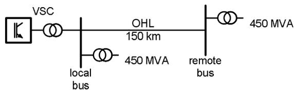
Moreover, there was a second 450 MVA transformer already connected to the local bus before the switching event and the transmission line was not compensated by a shunt reactor at the remote bus. Consequently the load flow conditions prior and after the energisation are not identical.
