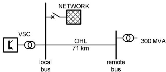
performed as a continuation of the above described soft-start test. The HVDC was feeding one of the two local bus bars while the other bus bar was still part of the integrated network. The bus coupling breaker was used to re-synchronize the isolated network. Primary voltage control was set to a 409 kV target value with a slope of 240 Mvar/kV, primary frequency control
