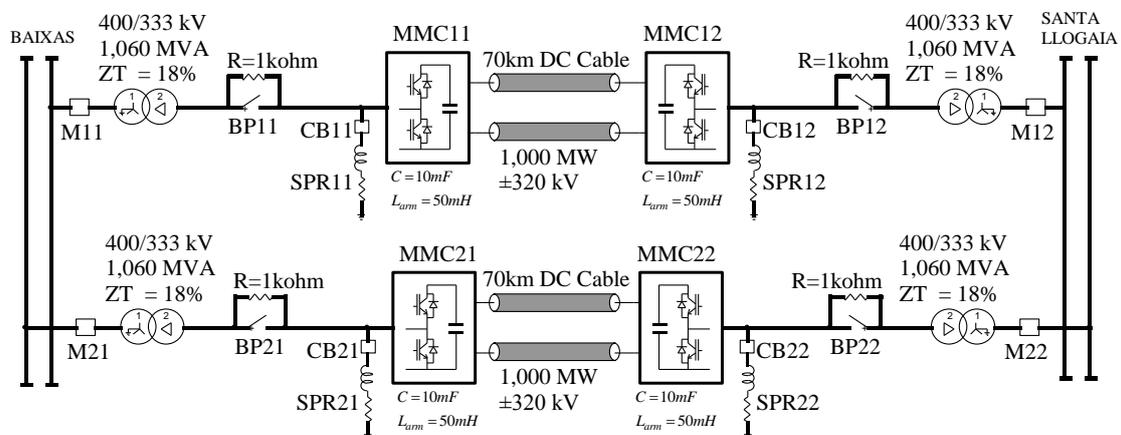
**Figure 2 : Single line diagram of INELFE interconnection**
