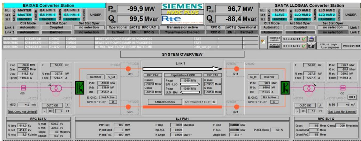
Figure 5: Replica and On-site HMI
