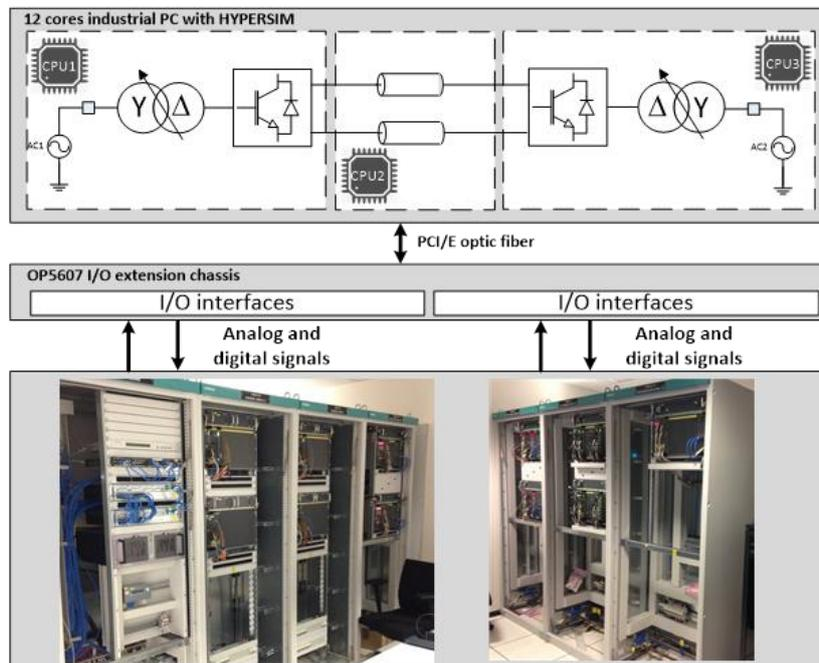
**Figure 4: HIL configuration of the INELFE Replica with Hypersim simulator**
