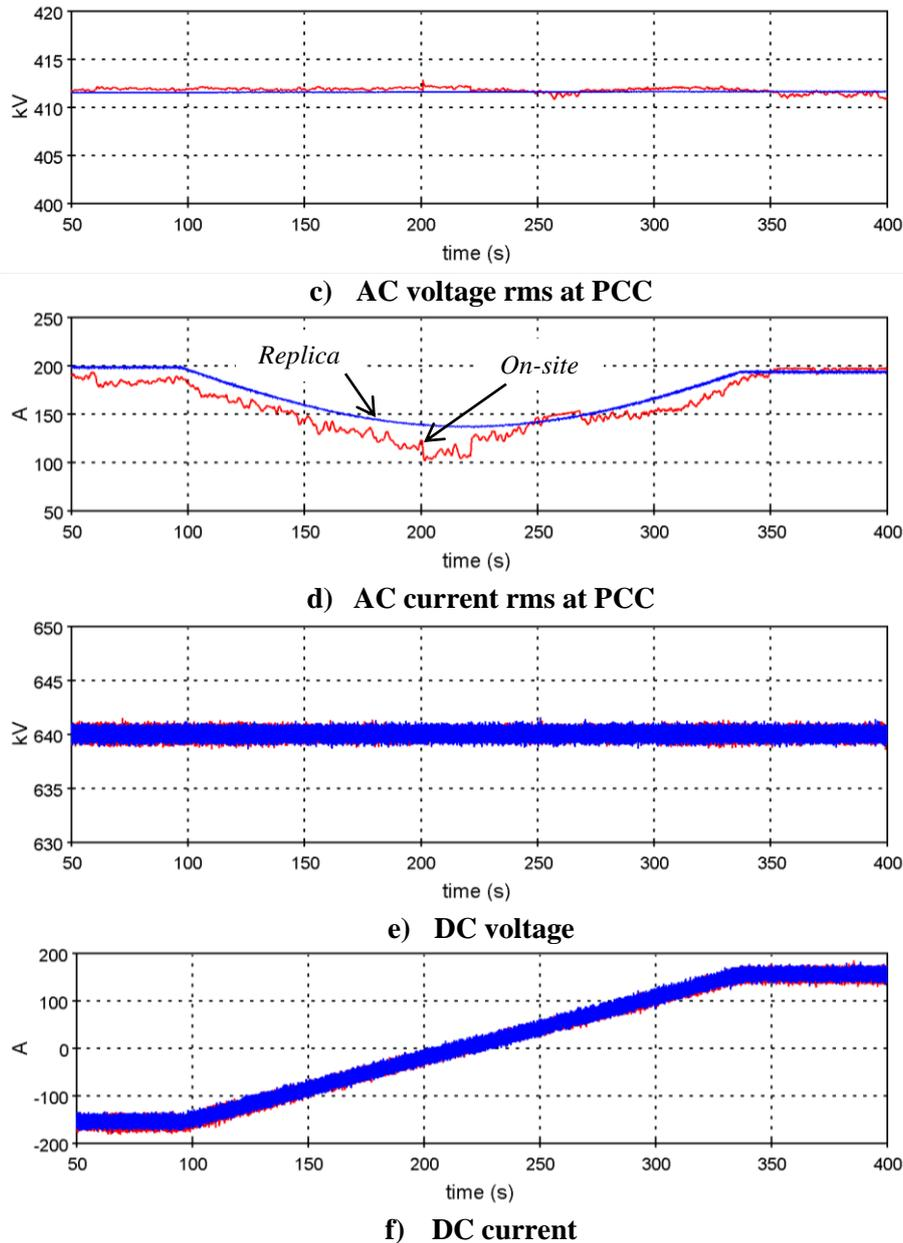
**Figure 6 : Comparaison between On-site and Replica results - variables at Baixas station**
