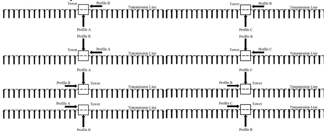
**Figure 8. All possible combinations of the vertical wind profiles (Load Case # 1 on the left and Load Case # 2 on the right) [15]**
