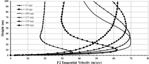
**Figure 2. Tangential velocity vertical profile at different distances ( $r$ ) from the center of the F2 tornado**
