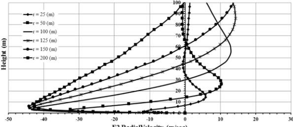
**Figure 3. Radial velocity vertical profile at different distances ( $r$ ) from the center of the F2 tornado**
