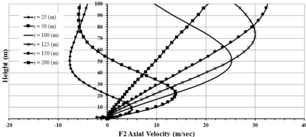
**Figure 4. Axial velocity vertical profile at different distances ( $r$ ) from the center of the F2 tornado**
