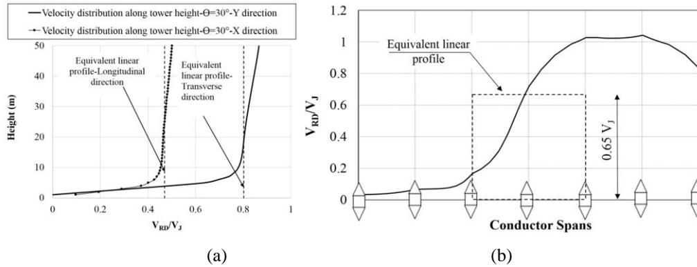
Figure 7 (a) Velocity distribution along tower height (b) Radial velocity distribution over six conductor spans
