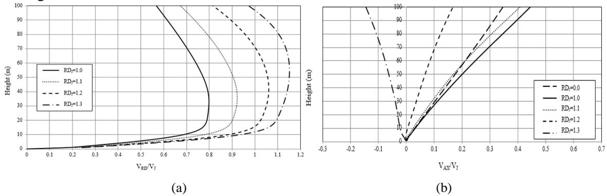
Figure 2 (a) Vertical profile of the horizontal/radial outflow wind speed,  $D_J=500$  m,  $\Theta=0^\circ$ , (b) Vertical profile of the axial outflow wind speed,  $D_J=500$  m,  $\Theta=0^\circ$  (El Damatty and Elawady [5])
