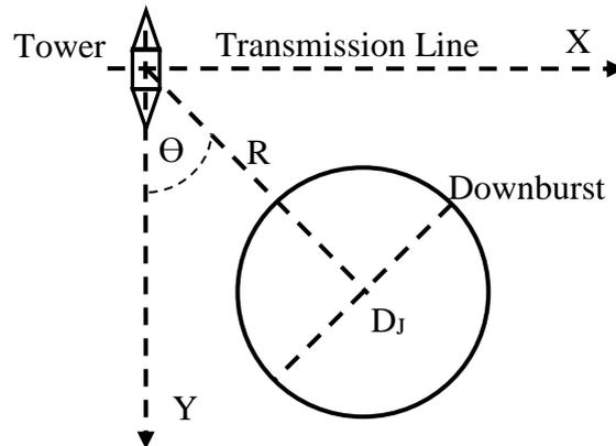
Figure 1 Downburst characteristics parameters
