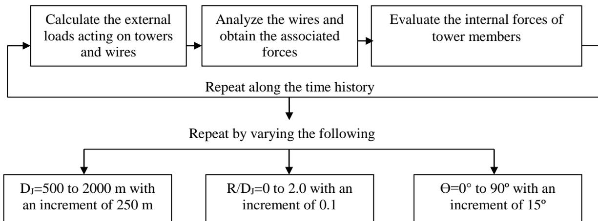
Figure 4 Flow chart summarizing the analysis steps conducted to obtain the downburst critical profiles
