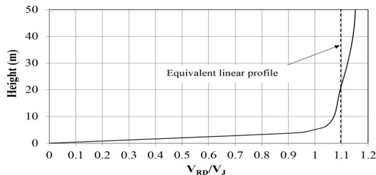
Figure 6 Velocity distribution along tower height
