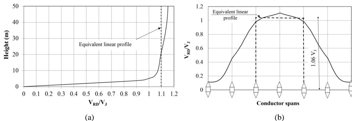
Figure 5 (a) Velocity distribution along tower height, (b) Velocity distribution over six conductor spans
