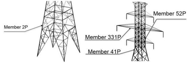
Figure 9 Self-supported tower T<sub>2</sub> selected members
