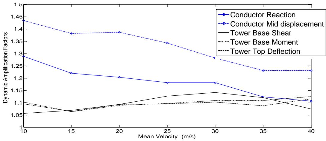
Figure 7 DAF for the H-frame steel TL
