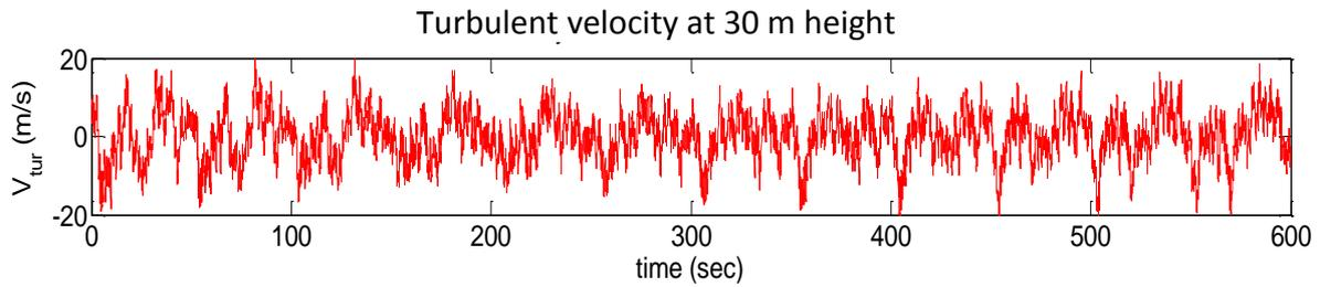
Figure 1 generated turbulent velocity for open terrain exposure
