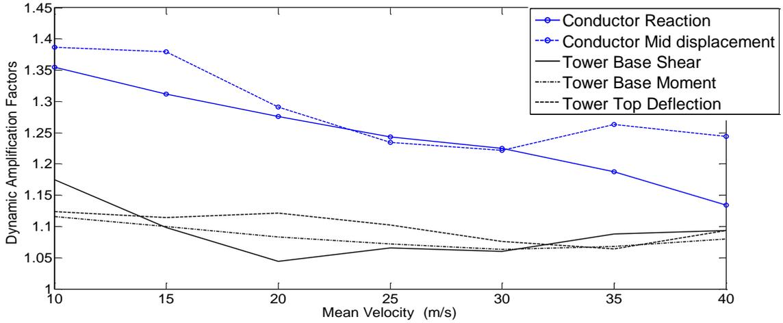
Figure 6 DAF for the self-supported tower
