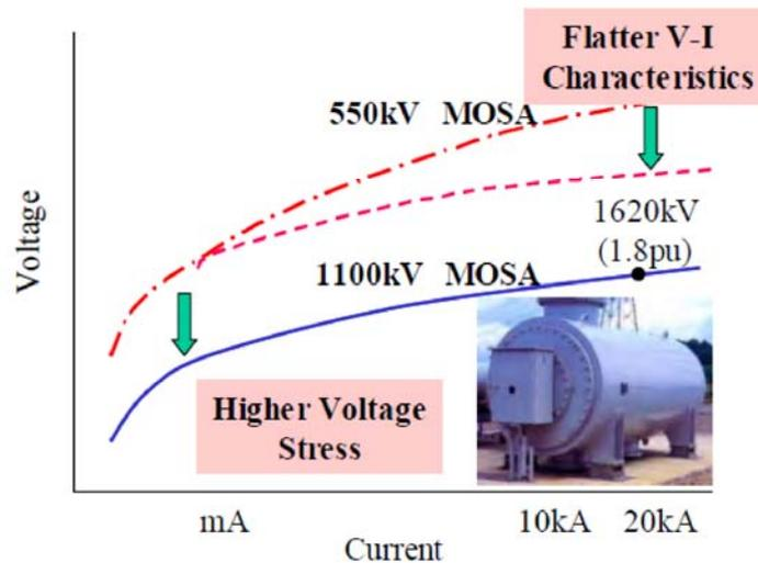
**Fig. 6.** Dead tank-type surge arrester with low protection level.
