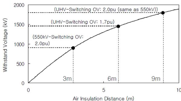
**Fig. 4.** Relation between air insulation distance and switching impulse withstand voltage.
