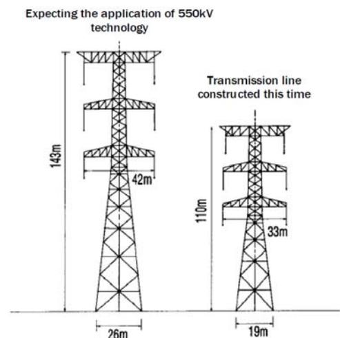
**Fig. 5.** Size reduction of 1100 kV double circuit tower,
