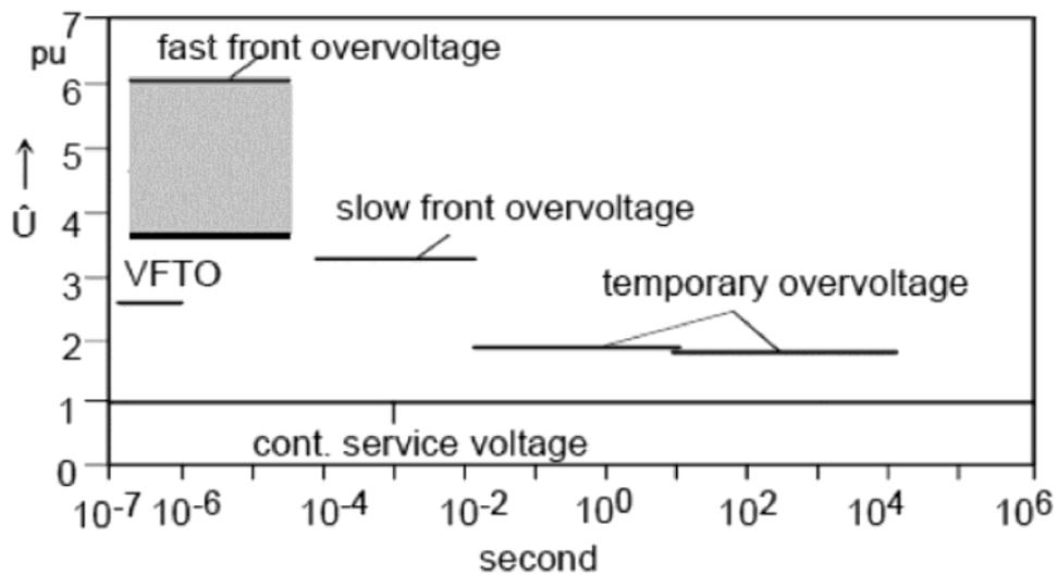
**Fig. 3.** Representative maxima of amplitude of overvoltages  $U_m$  (p.u.)
