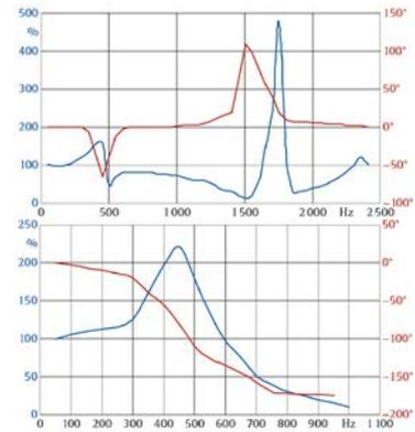
Figure 3: Relative output value and phase error of a MVT (top) and CVT (bottom) over signal frequency [2]
