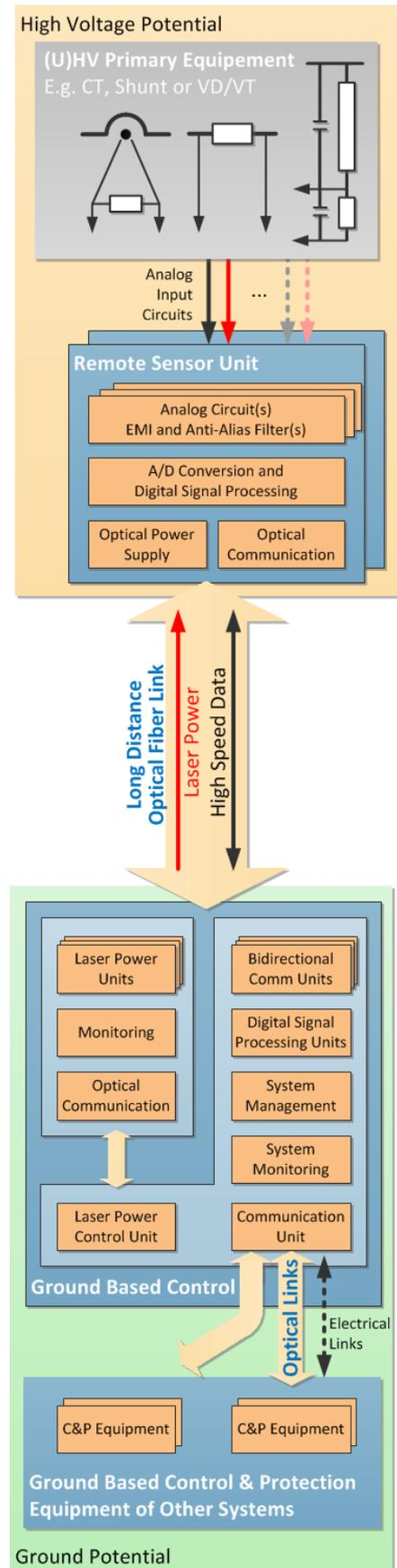
Figure 7: Illustration of the hybrid optical measuring solution HOM7 and system integration of other components
