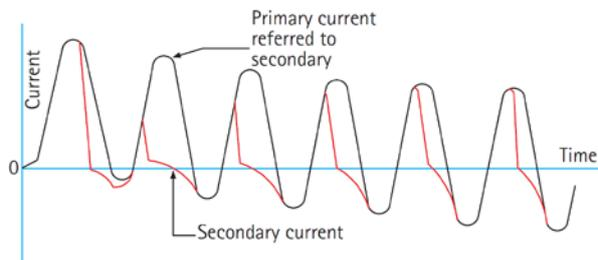
Figure 1: Transient condition at conventional CT [1]
