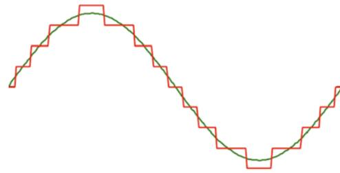
Figure 5: Illustration of principle of sinus approximation by MMC HVDC [3]
