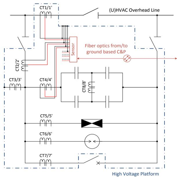
Figure 9: Typical single line diagram of SC installation
