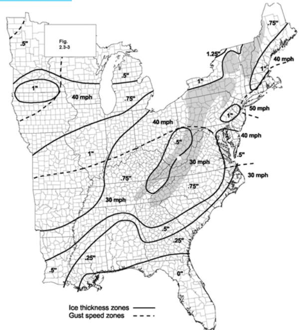
Figure 4 ASCE 10-05 ice with Concurrent Wind
