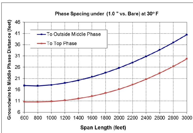
Figure 8 Phase Spacing between Groundwire and Middle Phase under Unequal Ice
