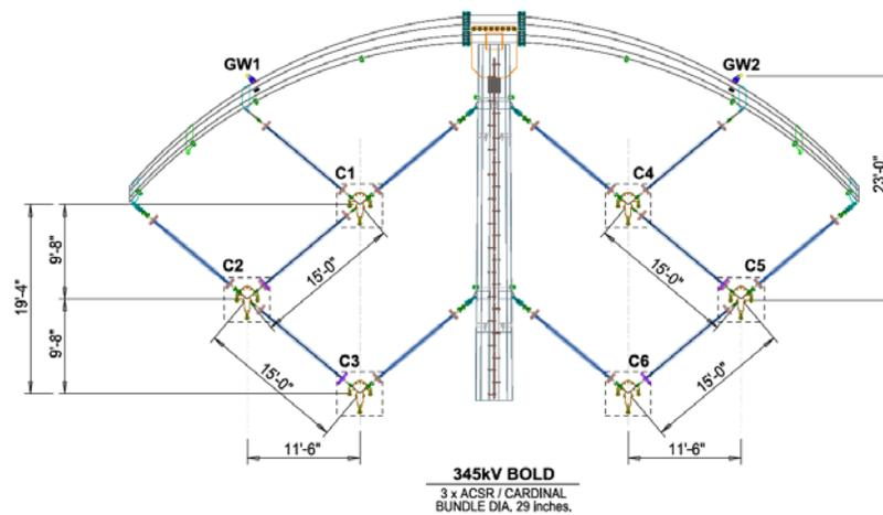
Figure 1 345 kV BOLD Phase Configuration
