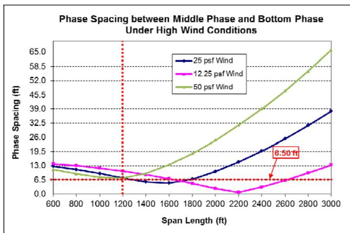
Figure 5 Phase Spacing under High Wind Conditions
