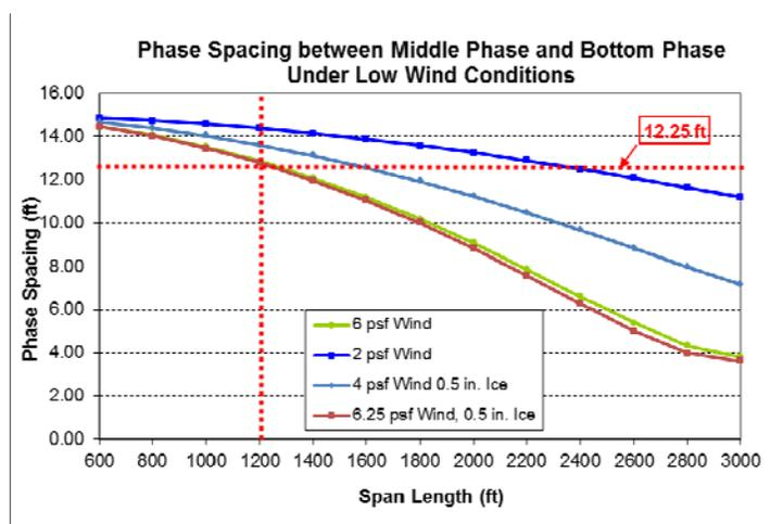
Figure 6 Phase Spacing under Low Wind Conditions
