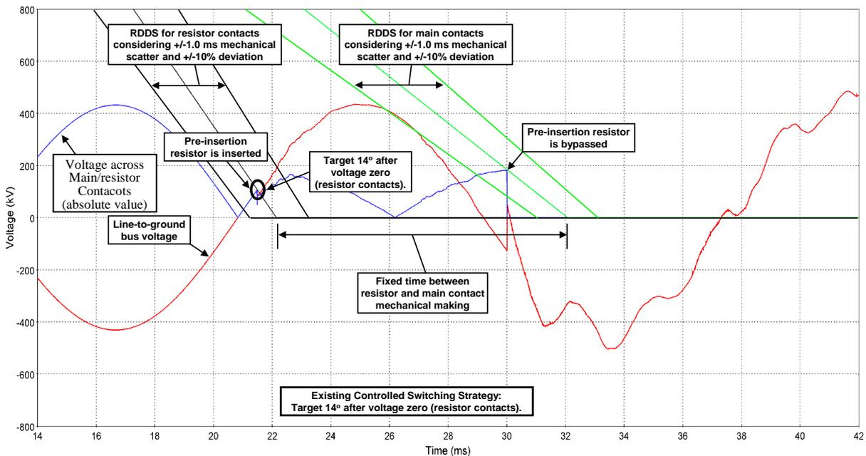
Figure 5 – Illustration of existing controlled switching strategy
