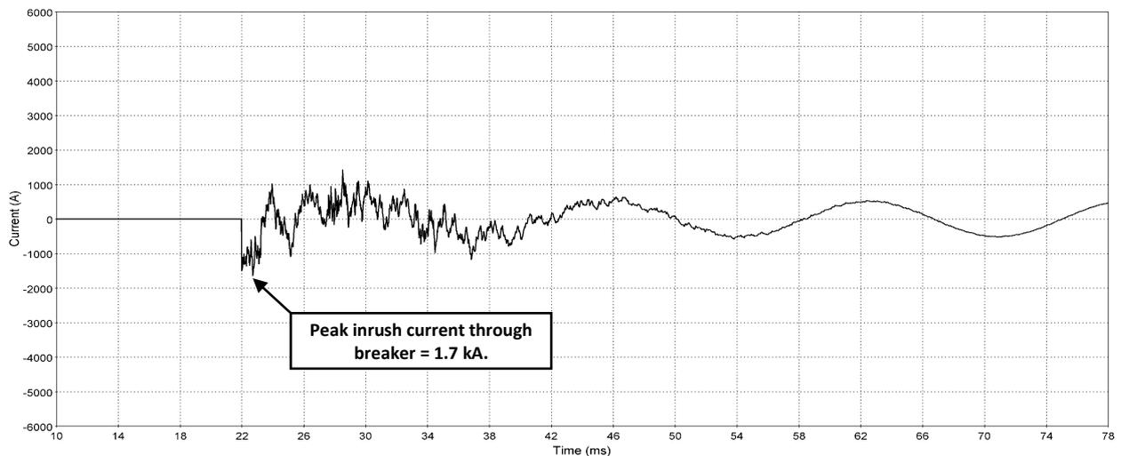
Figure 3 – Analysis of a close operation with only controlled switching
