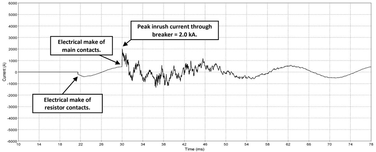
Figure 4 – Analysis of a close operation with the original controlled switching target
