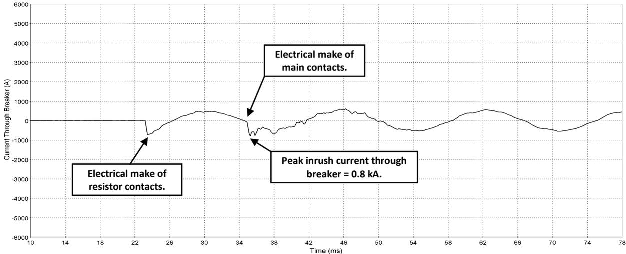
Figure 9 – Measured close operation with new controlled switching target
