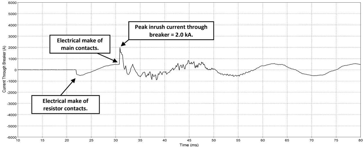
Figure 8 – Measured closing operation with original controlled switching target
