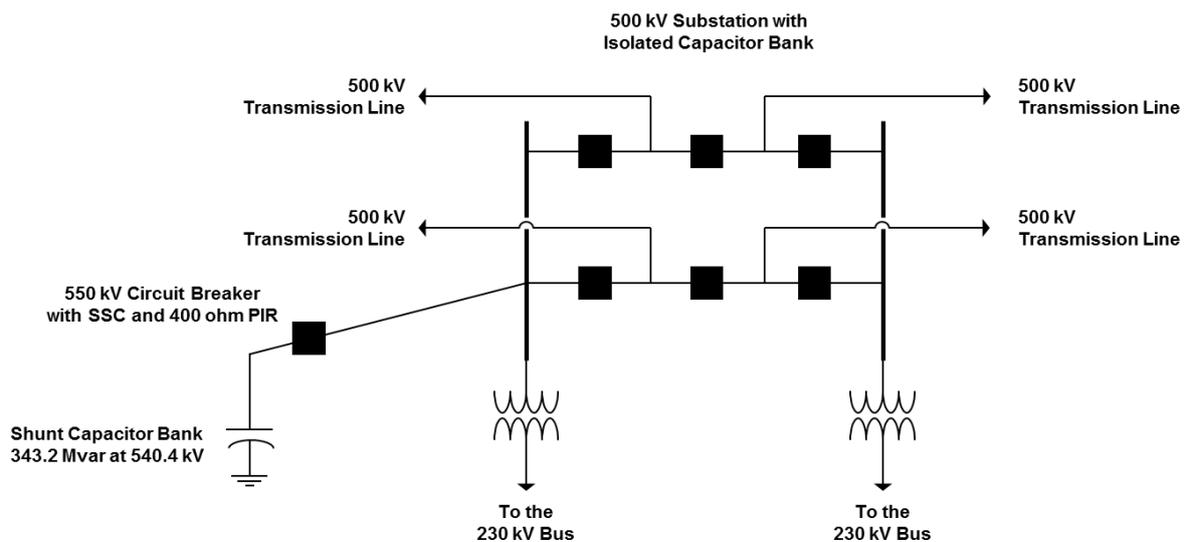
Figure 1 – One-line diagram
