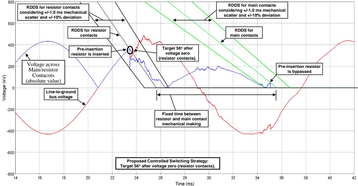
Figure 6 – Illustration of proposed controlled switching strategy
