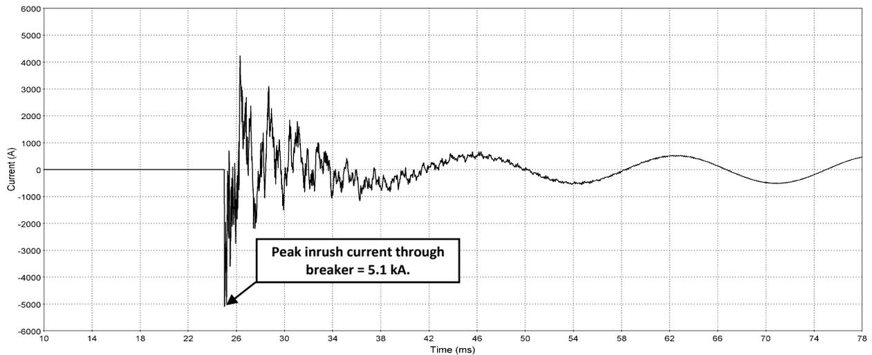
Figure 2 – Analysis of a close operation without controlled switching and closing resistors
