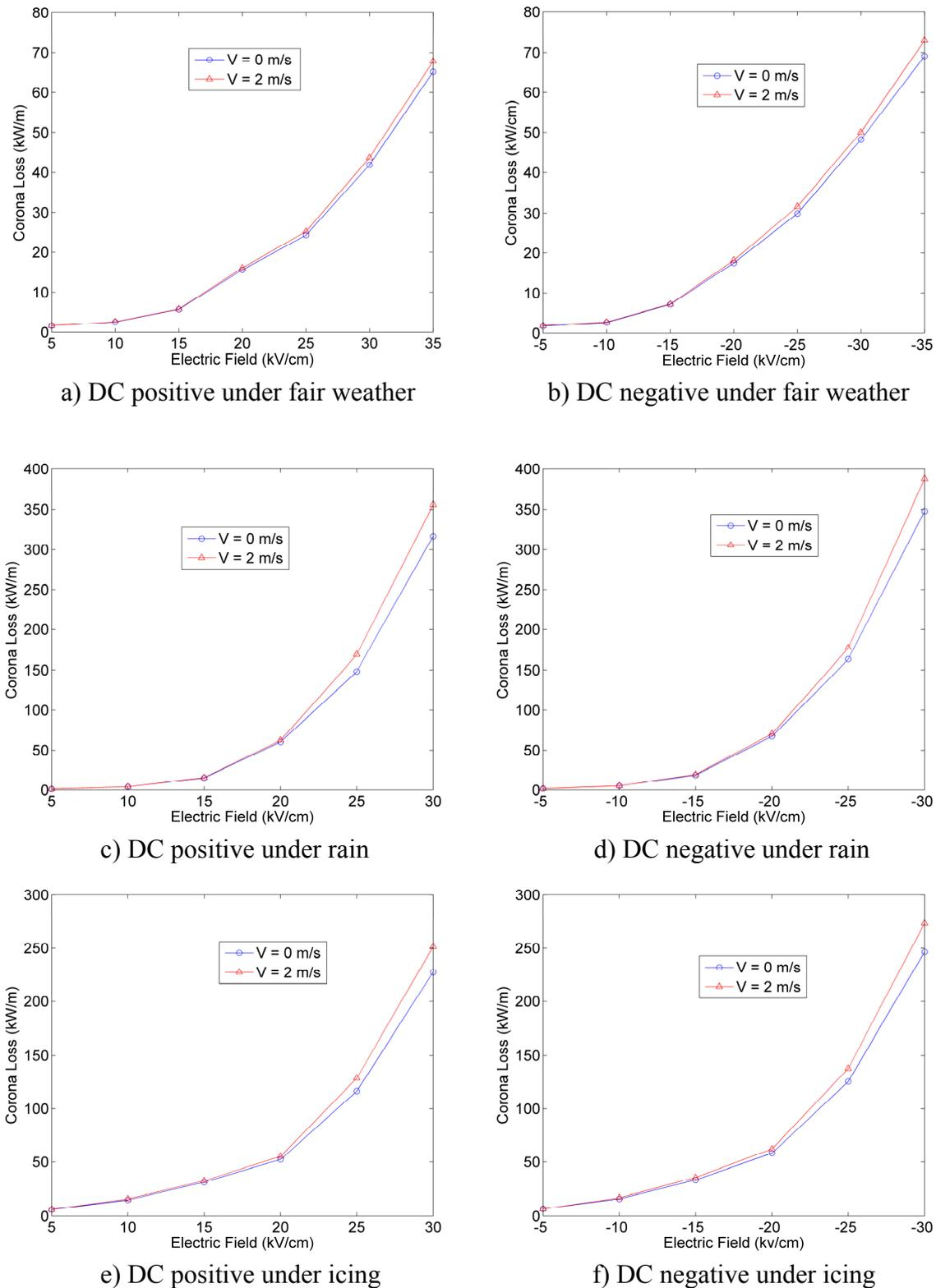
Fig. 4. Corona loss vs. electric field strength under DC voltages
