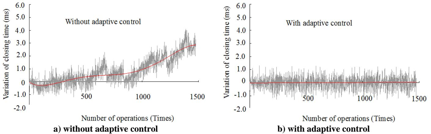
**Figure 6: Typical drifts of the closing time measured with and without adaptive control**
