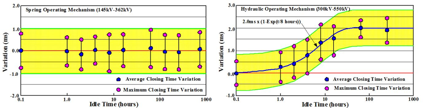
Figure 3: Idle time influence: comparison between spring and hydraulic operating mechanisms
