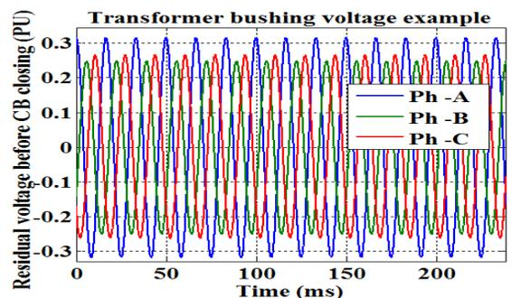
**Figure 7: Example of coupling voltage on the transformer due to capacitive voltage divider formed by the grading capacitors and the load**
