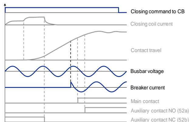
**Figure 5: Typical recorded signals during commissioning**
