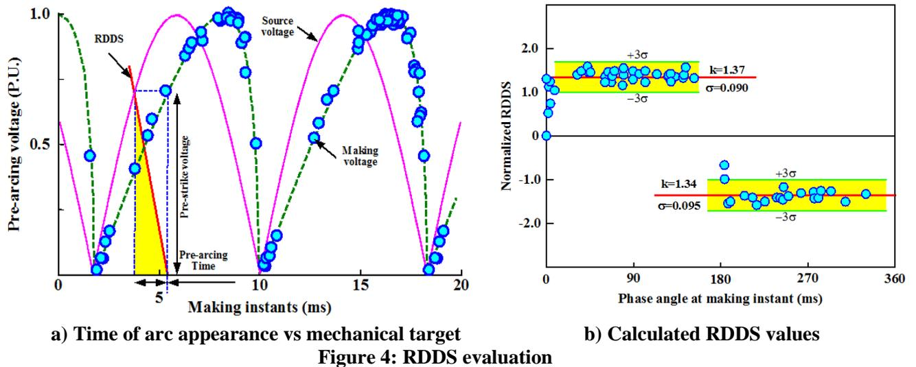
The CSD can only control the CB to make/separate the main contacts at a programmed instant (mechanical target). Therefore, the RDDS value must be calculated properly and configured in the CSD to enable it to work optimally by converting the required electrical target (i.e. what the system and the engineer need) into a mechanical target (i.e. what is needed by the CB control coil).
