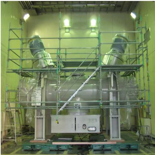
Fig. 4. 800 kV GCB during high and low temperature test
