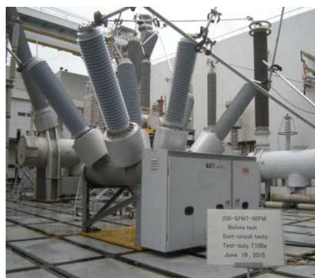
Fig. 6. 245 kV mixed gas GCB during interruption test
