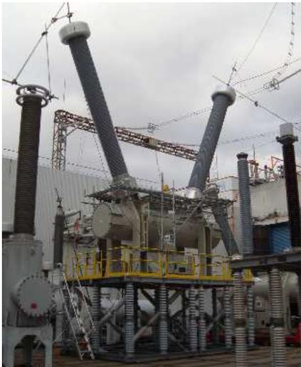
Fig. 3. 800 kV GCB during interruption test
