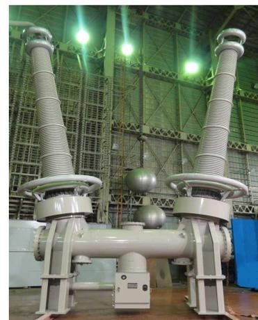
Fig.12. 550kV Torsion bar spring operated GCB
