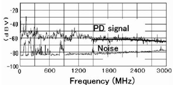
Figure 1 Spectra of electromagnetic waves of PD radiated from insulating spacer
