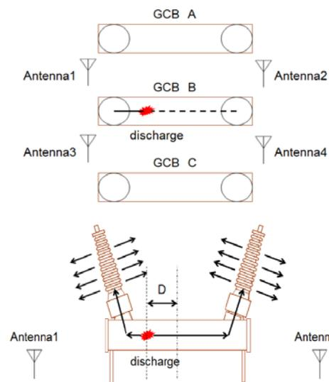
Figure 11 Location of four antennas for dead tank GCB
