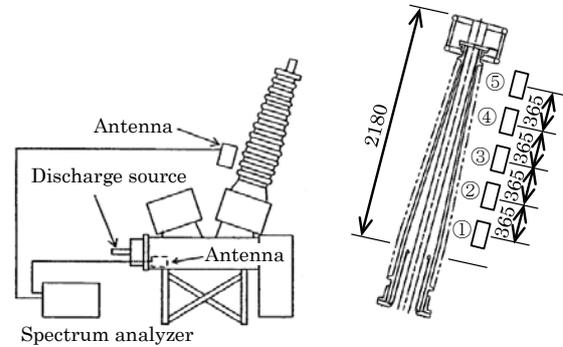
Figure 9 Experimental set-up and measurement point for electromagnetic wave
