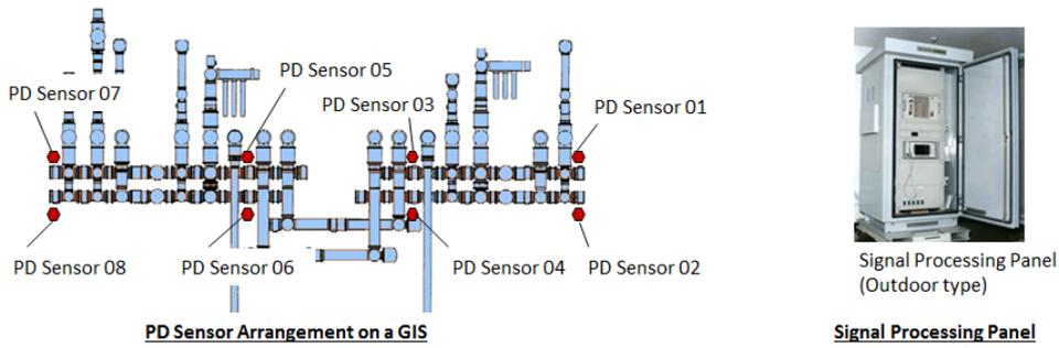
Figure 6 Online partial discharge monitoring and diagnosis system
