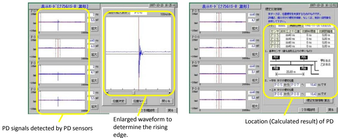
Figure 7 Screenshot of the HMI display for partial discharge location
