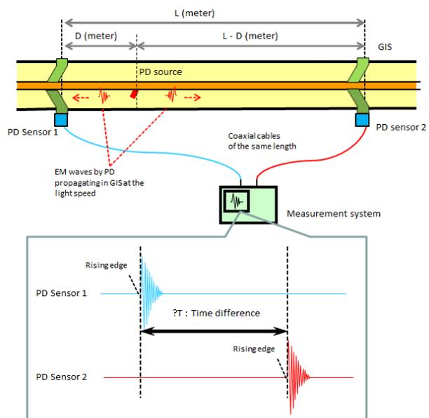
Figure 8 Principle of PD location
