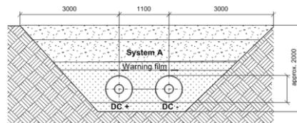
**Fig. 11:** Space required for 5 GW power transmission at 500 kV DC
