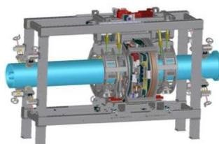
Fig. 10: New jointing technology based on friction steer welding
