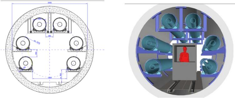
**Fig 3:** Bored tunnel for two three phase AC systems up to 550 kV and 4000 MVA power transmission
