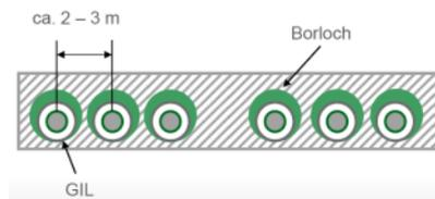
**Fig. 5:** Directly buried GIL for two three phase AC system up to 550 kV and 4000 MVA power transmission
