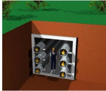
**Fig. 4:** Squared tunnel for two three phase AC systems up to 550 kV and 4000 MVA power transmission
