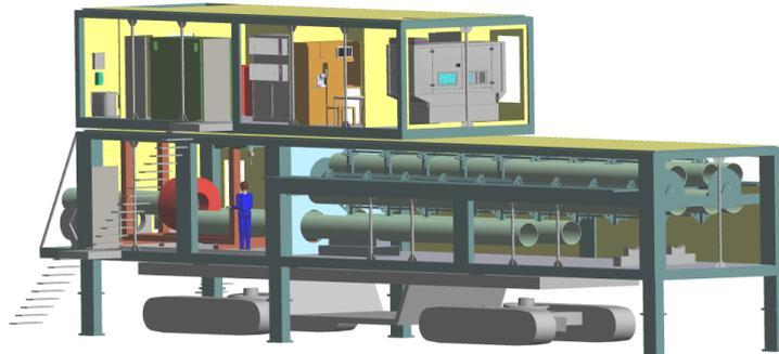
Fig. 9: Mobile factory for on-site assembly and laying
