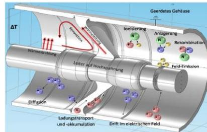
**Fig. 13:** Physical principles of DC gas-insulated systems
