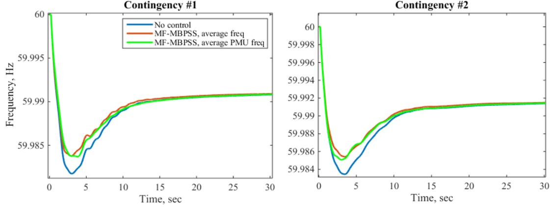
Fig. 2. Impact of MF-MBPSS control on frequency response
