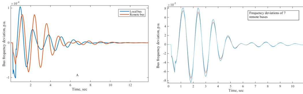
Fig. 5. System response to a pulse signal: A – local vs. remote; B – remote buses coherency
