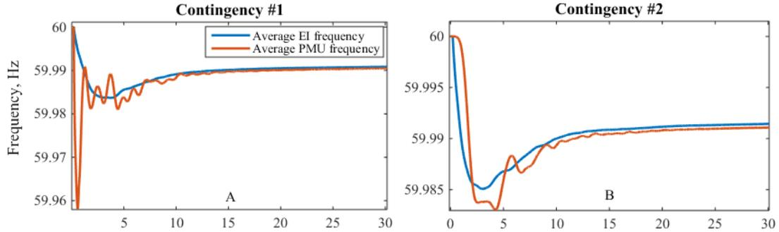
Fig. 1. EI frequency response: dependence of PMU measurements on outage location
