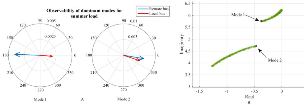
Fig. 6. Signals' properties: A – modes observability; B – root locus with applied feedback for remote signal
