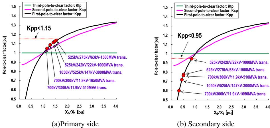
Figure 5: Typical evaluations of first-pole-clear factor ( $K_{pp}$ ) for TLF conditions
