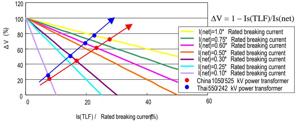
Figure 3: Voltage drop across the transformer( $\Delta V$ ) for various values
