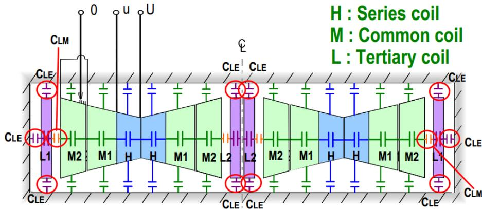
Figure 11: Cross sectional diagram of the transformer coil
