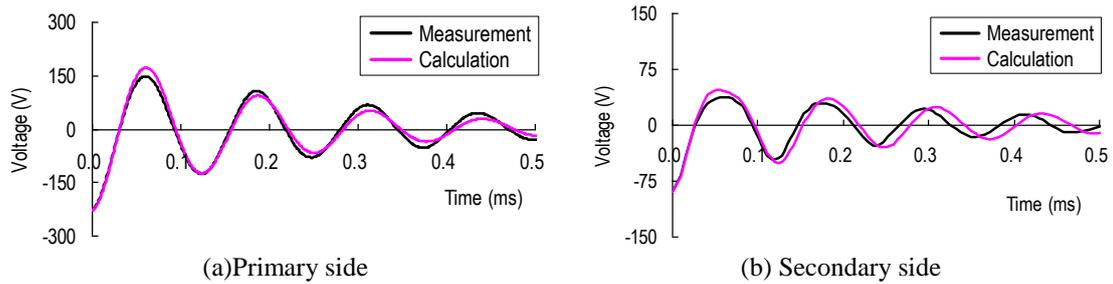
Figure 10: TRV reproduced by simplified transformer models
