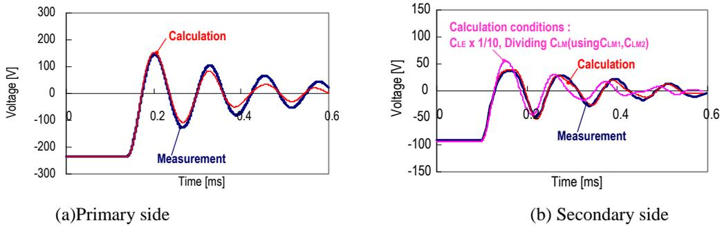
Figure 13: TRV reproduced by the manufacturer transformer model
