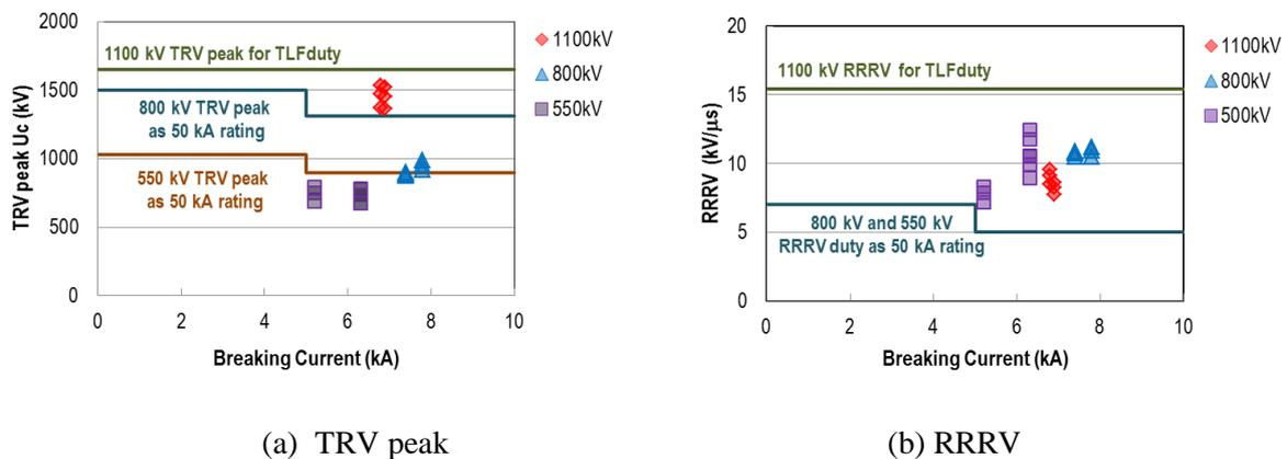
Figure 6: TRV for TLF conditions at primary side of transformer
