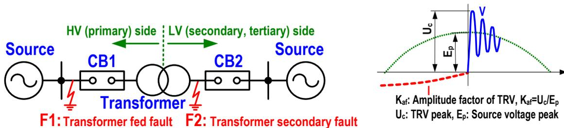
Figure 1: Transient Recovery voltage (TRV) for Transformer limited Faults (TLF)
