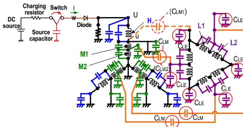
Figure 12: Manufacturer transformer model with five elements model for three-phase autotransformer 525/275/63 kV, 1500 MVA
