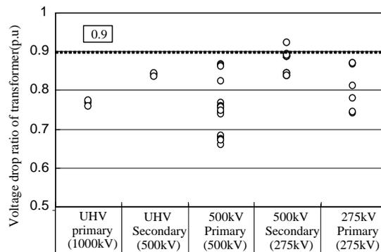
Figure 4: Examples of voltage drop ratio of EHV and UHV power transformers
