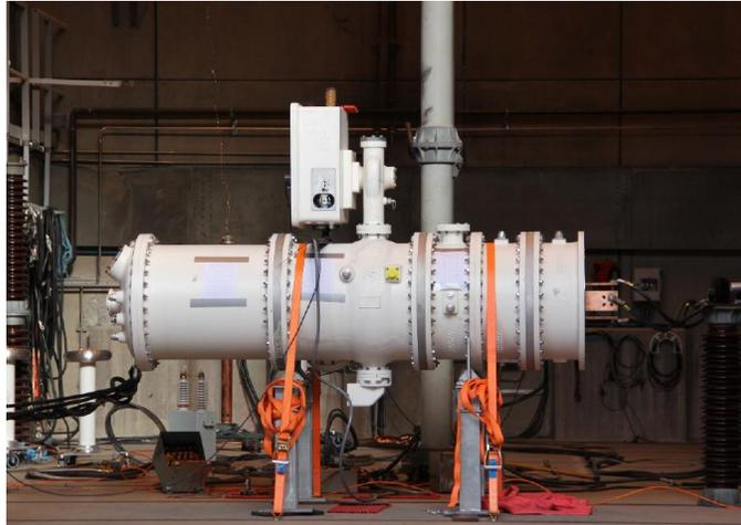
Figure 2 FAES assembled for making test
