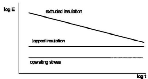
Fig 2 Lifetime curve for extruded cable insulation
