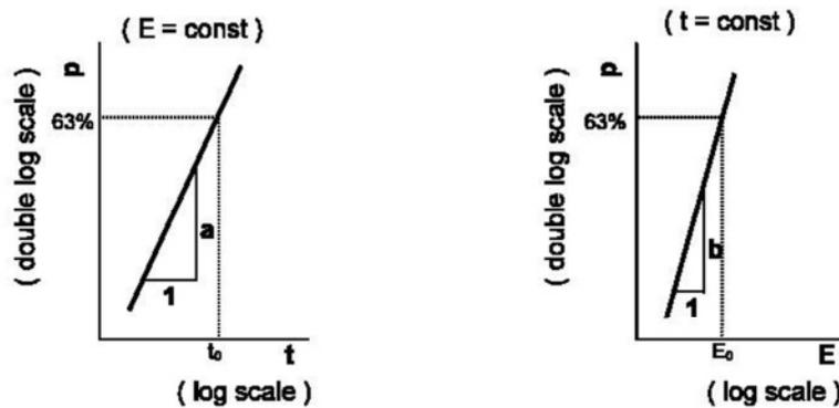
Fig 1: Partial Weibull distributions of breakdown time (constant stress) and stress (constant time) for an extruded cable insulation
