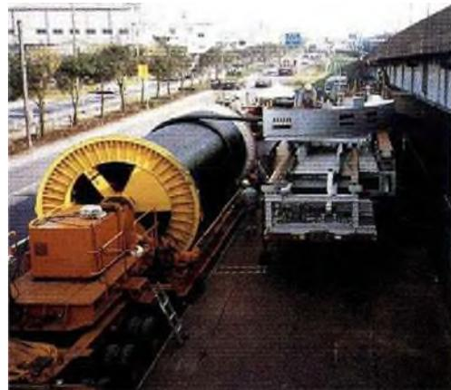
**Fig 7: Drum of 500 kV 2500mm<sup>2</sup> XLPE Cable**
