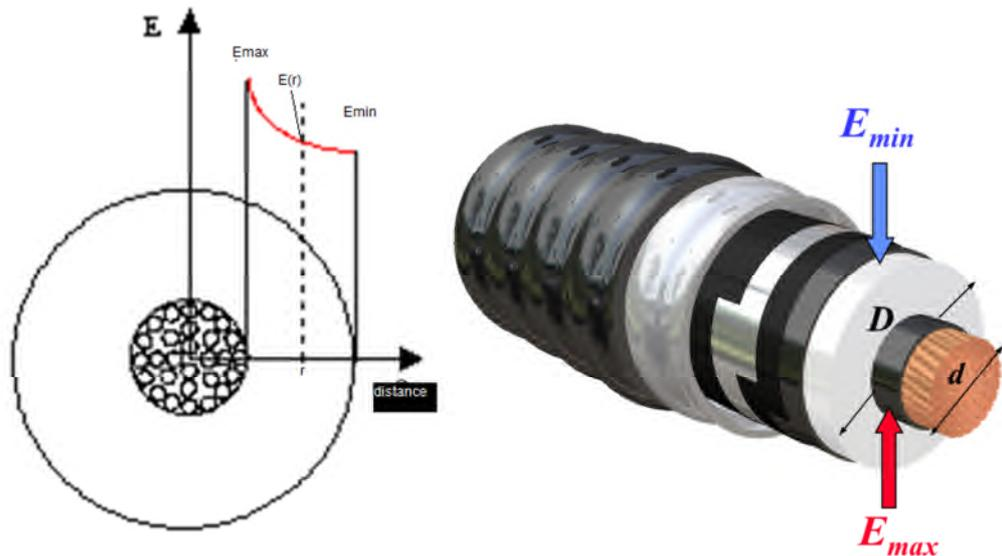
$E_{max}$  is very important for the ageing of the insulation and the performance of the cable under impulse.
