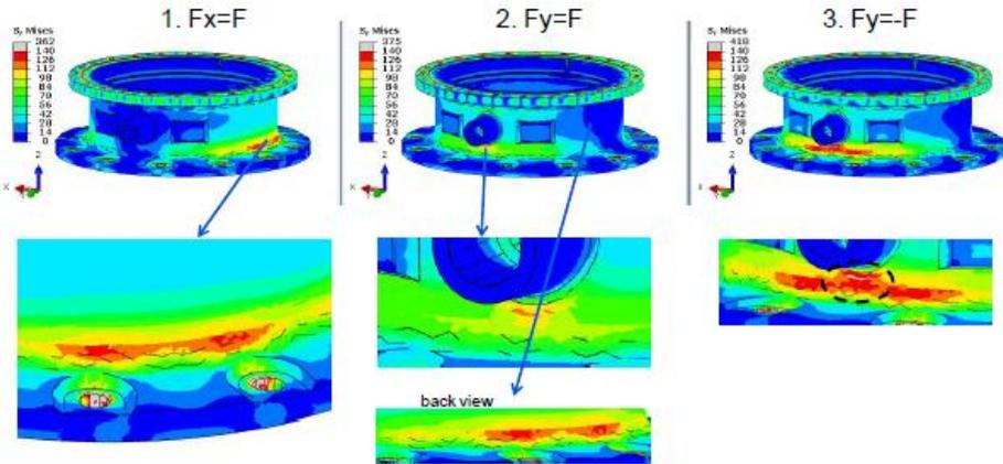
Figure 3. Details from the FEM analysis for the mounting flange
