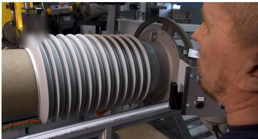
Figure 2. Manufacture of outer insulation.
