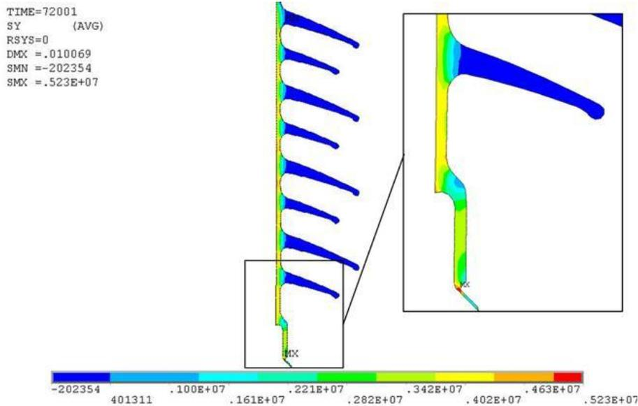
Figure 5. FEM calculation of silicone sheds
