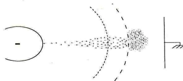
Fig. 1: Ionic current flow of a unipolar HVDC transmission line.
