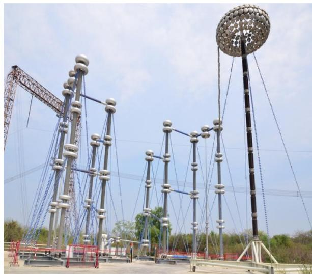
Fig. 8: View of  $\pm 1200$  kV HVDC source
