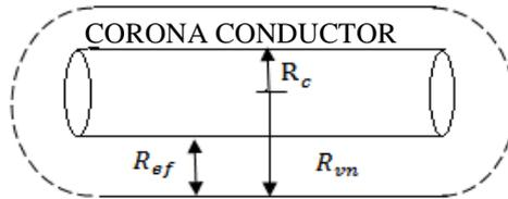
Fig. 2: Ionization region formation around the HVDC conductor.
