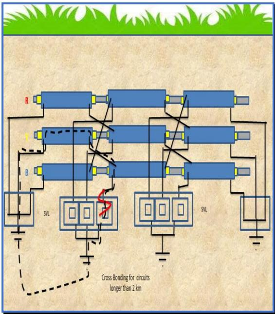
Fig-10, Fault Current in Cross Bonding
