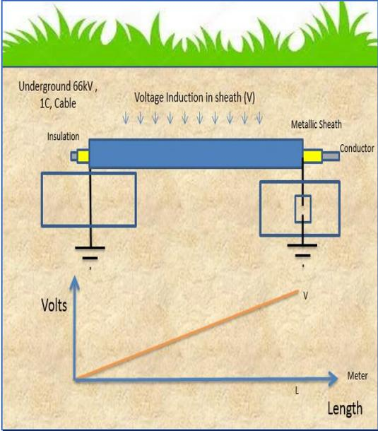
Fig-4, Single Point Bonding
