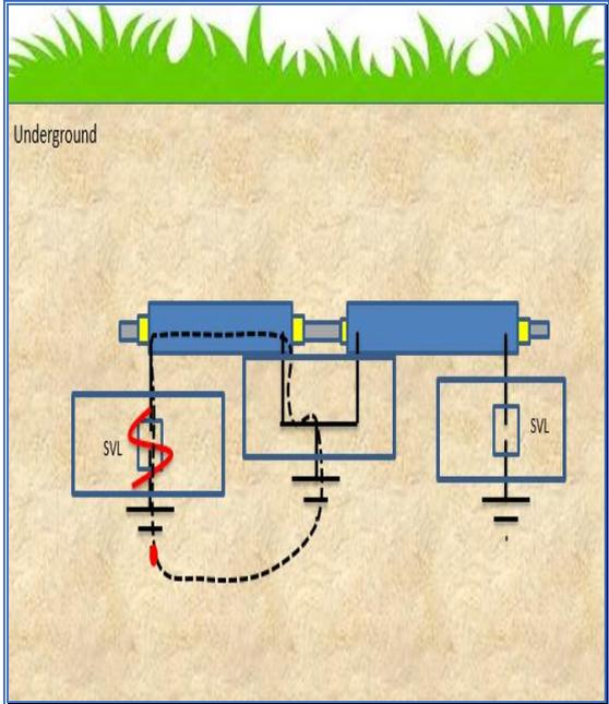
Fig-9, Fault current in Single Point Bonding
