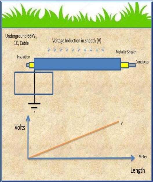
Fig-3, Un-bonded cable
