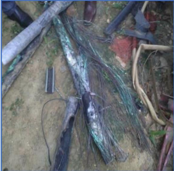
Fig-7, Damaged Cable
