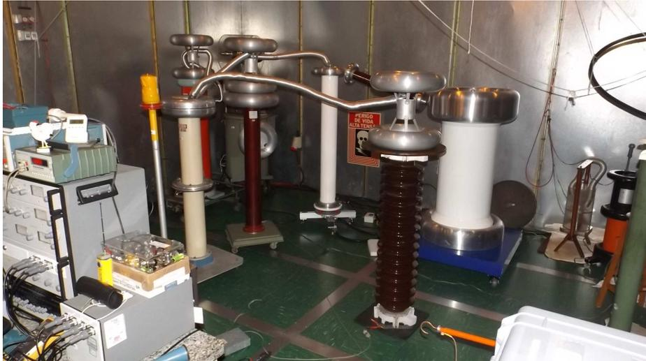
**Figure 10 – Arrangement in the laboratory for PD measurement on the surge arrester module**
