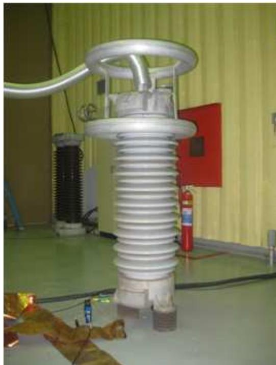
**Figura 3 – Lab test circuit to evaluate the sensitivity of HFCT**
