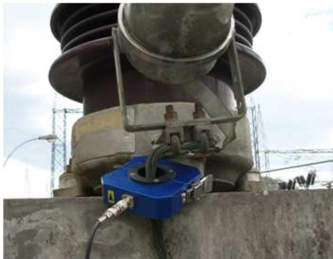
**Figure 1 – Clamp HFCT on the grounding cable of a surge arrester**
