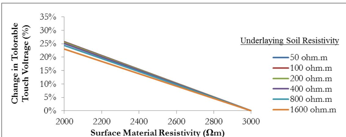
Figure 5- Tolerable Touch Voltage vs. Surface Material Resistivity
