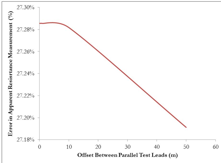
Figure 7- Error in Resistance Measurement Due to Proximity between the Test Leads
