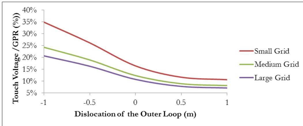
Figure 3- Touch Voltage as a factor of GPR vs. Ground Grid Outer Loop Dislocation
