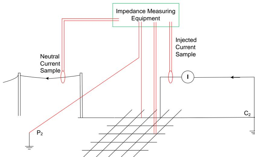
Figure 6- Modified Fall-of-Potential Test Method [4]
