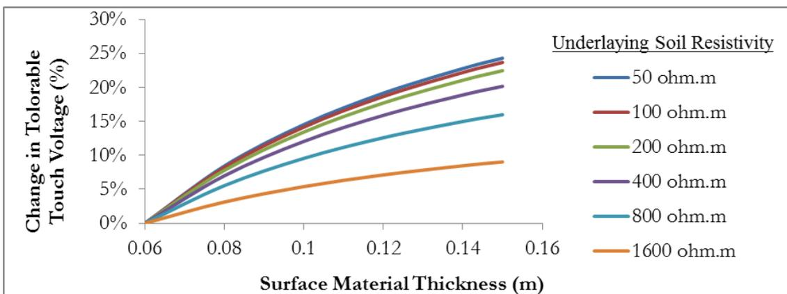
Figure 4- Tolerable Touch Voltage vs. Surface Material Thickness
