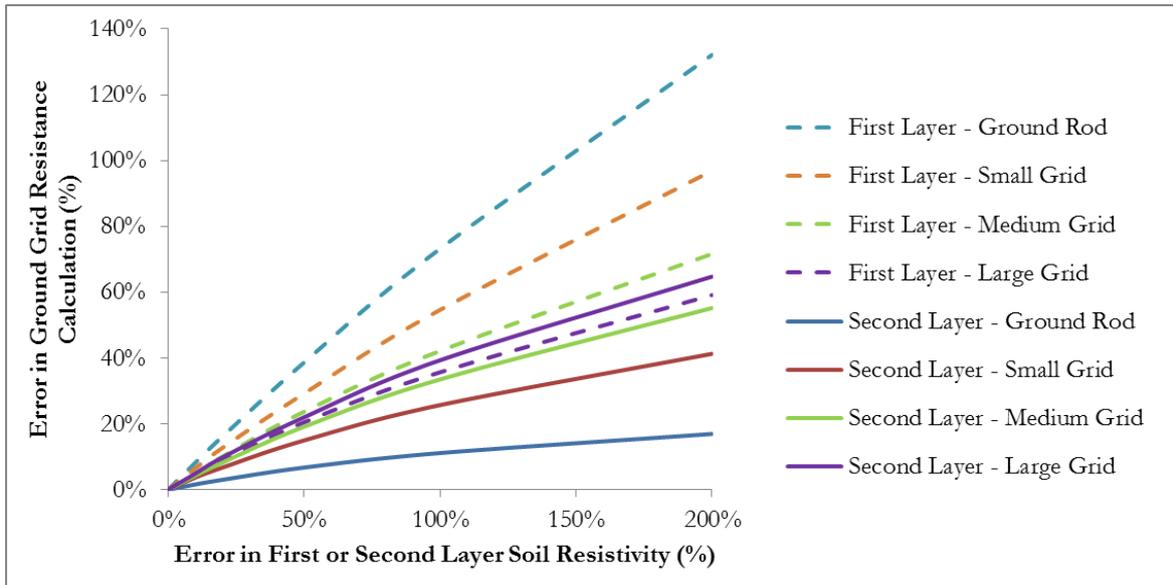
Figure 2- Error in Ground Grid Resistance (Unreliable First or Second Layer Soil Resistivity)
