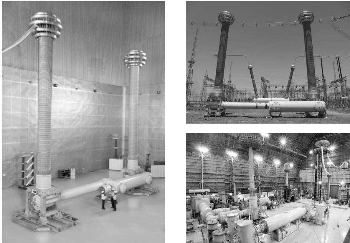
Figure 1 1200 kV mixed technology switchgear for new UHV grids in India, dielectric type tests (left), 1200 kV mixed technology switchgear for new UHV grids in India, on-site tests (right, at the top), dielectric test setups of 1100 kV CB in Japan (right, at the bottom)
