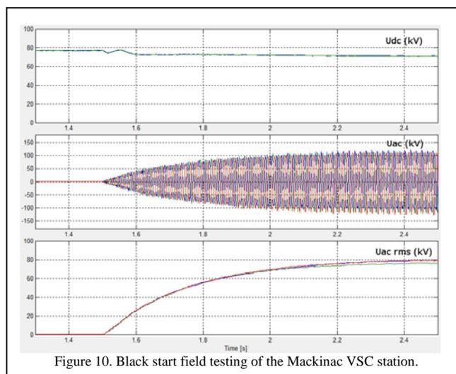
Figure 10. Black start field testing of the Mackinac VSC station.
