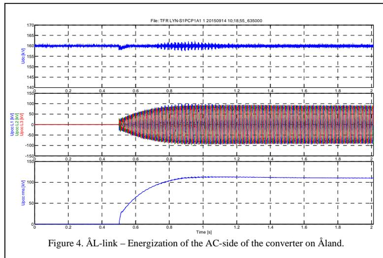
Figure 4. ÅL-link – Energization of the AC-side of the converter on Åland.
