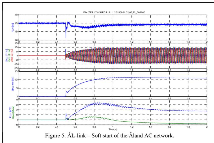
Figure 5. ÅL-link – Soft start of the Åland AC network.
