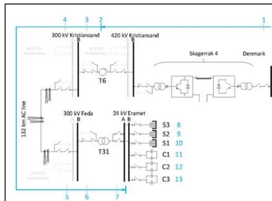
Figure 7. Black-start test grid, the blue numbers corresponds to order of connection.
