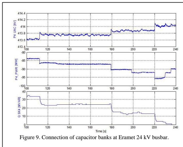
Figure 9. Connection of capacitor banks at Eramet 24 kV busbar.
