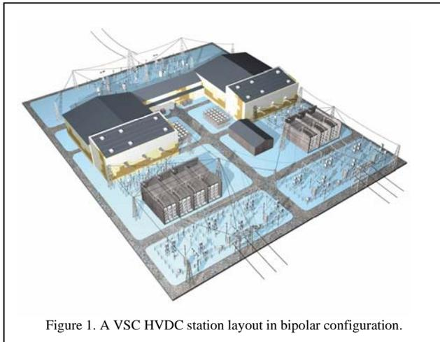
Figure 1. A VSC HVDC station layout in bipolar configuration.
