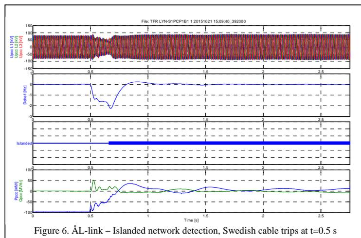
Figure 6. ÅL-link – Isolated network detection, Swedish cable trips at t=0.5 s
