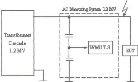
Figure 7. Electrical scheme for AC test.
