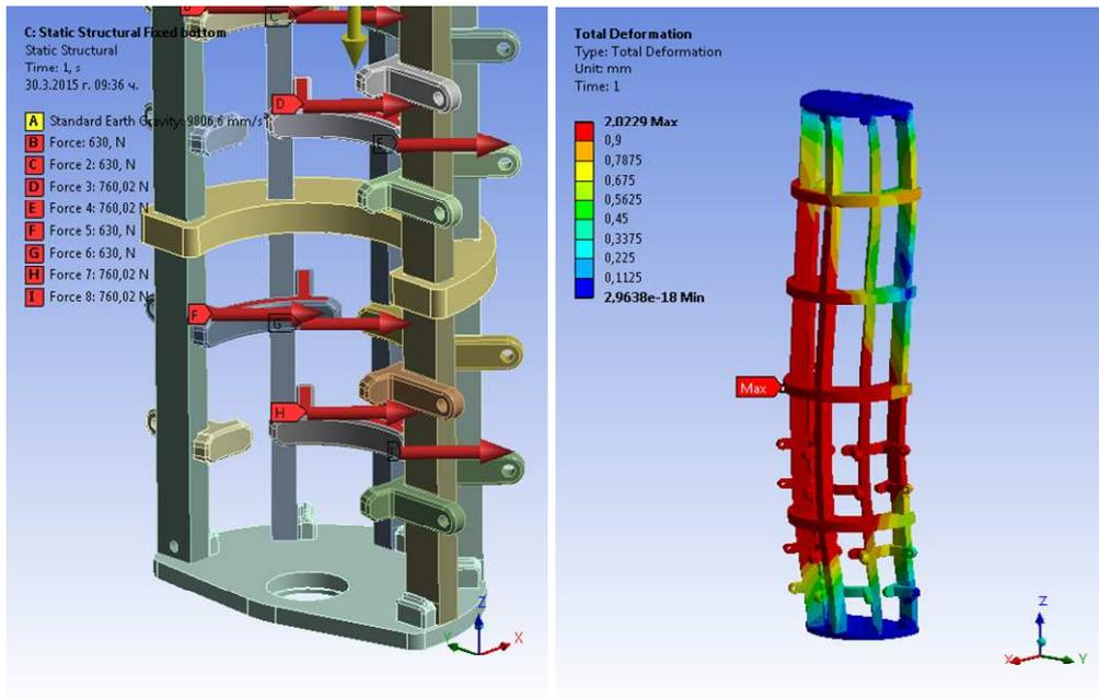
Figure 6. Total deformation during short circuit.
