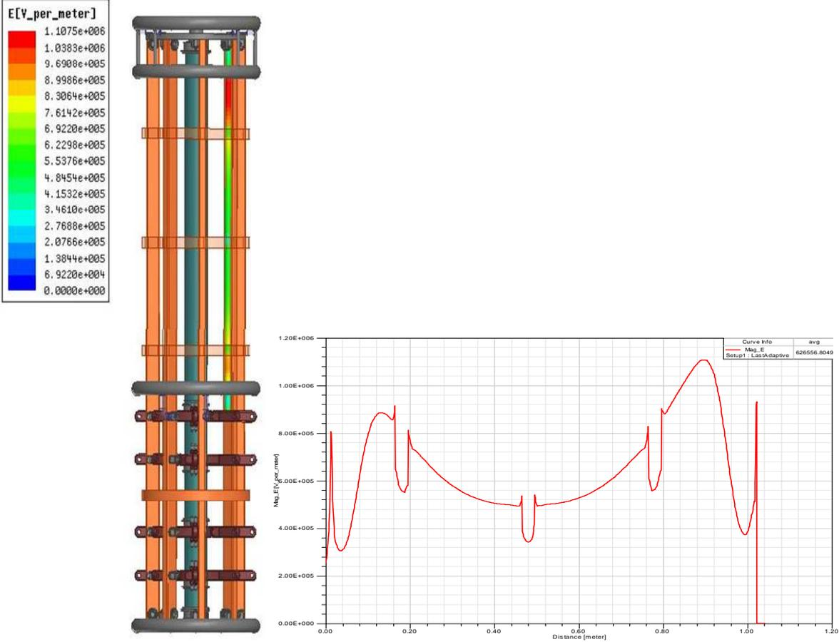
Figure 5 Field Stress along insulation bar.
