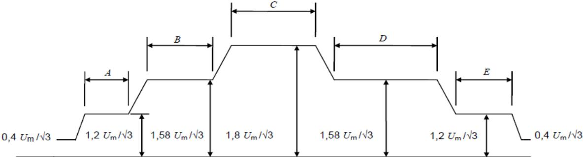
Figure 8. Time sequence for the application of test voltage (de-energized tap-changer) [1]
