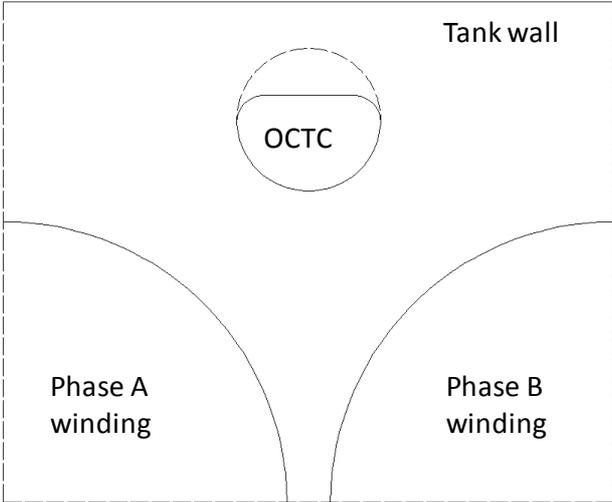
Figure 1. Schematic arrangement of OCTC and winding in transformer tank
