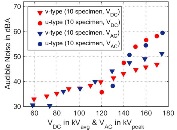
**Figure 5: Difference in hissing and crackling audible noise for AC & DC voltage**
