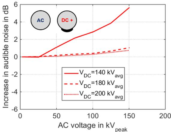
**Figure 6: Effect of a pure AC ripple (Case 1a) on DC AN for different DC voltages**
