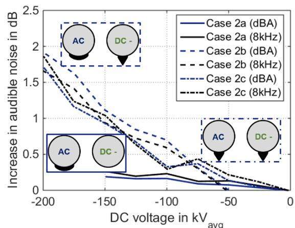
**Figure 9: Impact of DC corona (Case 2b & 2c) on AC AN in comparison to a pure DC bias (Case 2a),  $V_{AC} = 180$  kV<sub>peak</sub>**
