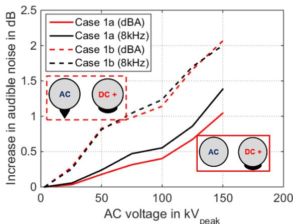
**Figure 8: Impact of AC corona (Case 1b) on DC AN in comparison to a pure AC ripple (Case 1a),  $V_{DC} = 180$  kV<sub>avg</sub>**
