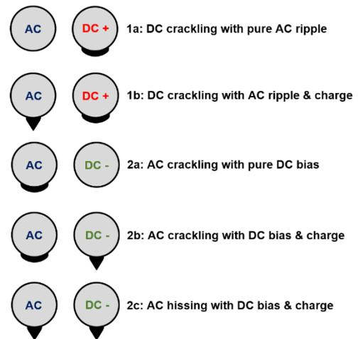
**Figure 3: Hybrid test cases using artificial defects as corona sources**
