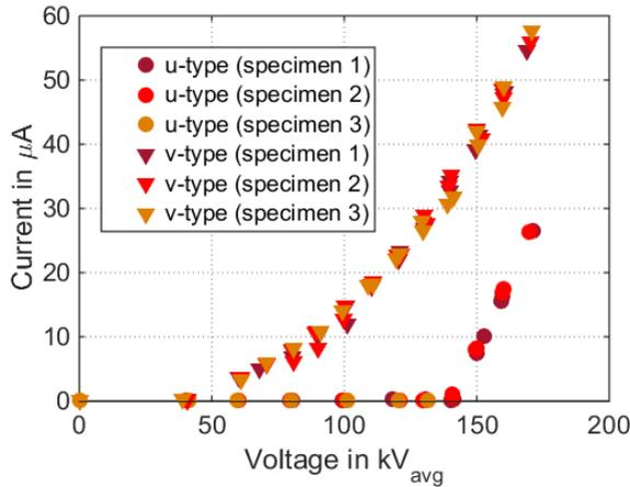
**Figure 4: Reproducibility of DC corona current for the different specimen and shapes**
