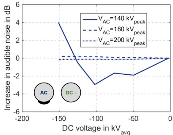
**Figure 7: Effect of a pure DC bias (Case 2a) on AC AN for different AC voltages**
