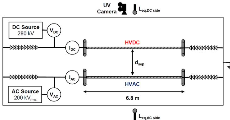
Figure 1: Hybrid AC/DC test setup
