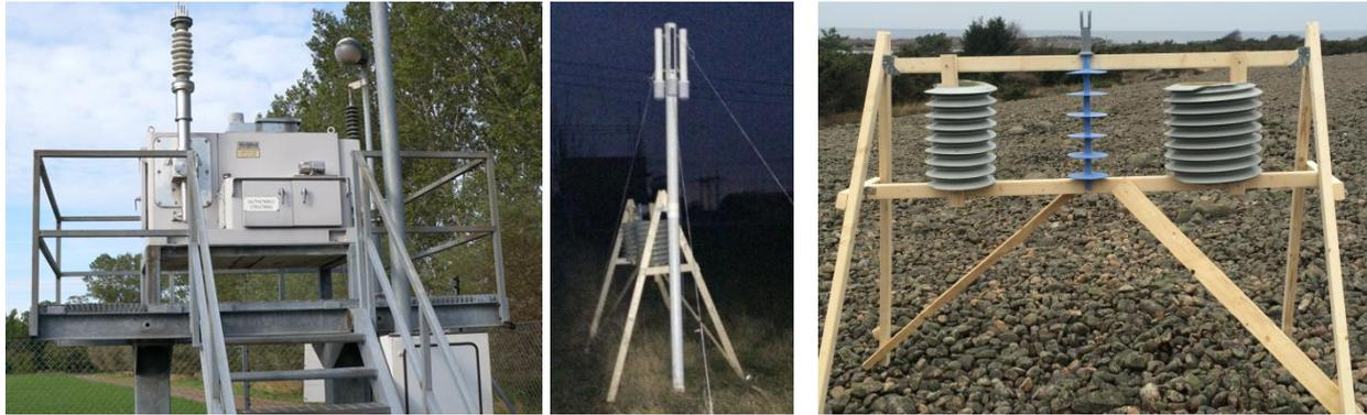
Figure 2 Left: Automatic Pollution Monitor; Middle: Dust Deposit Gauge; Right: de-energized test station for pollution/hydrophobicity measurements on composite insulators with different diameters.
