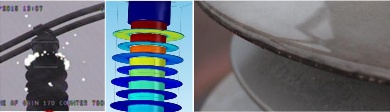
Figure 5 Left: corona observed in service; Middle: too high E-field leading to corona in service and loss of hydrophobicity; Right: reduction of hydrophobicity close to the high-voltage ends in service.
