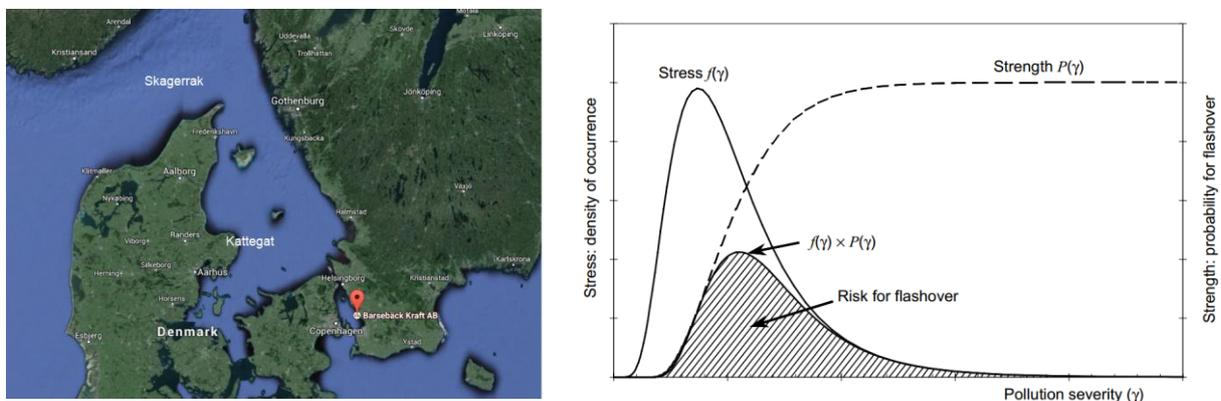
Figure 1 Left: location of Barsebäck substation (red marker); Right: principles of statistical dimensioning according to Annex G of IEC 60815-1 [2].
