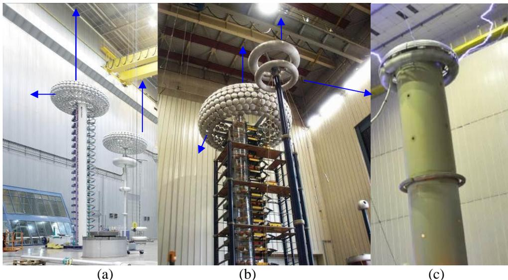
Figure 2. (a) and (b) Impulse generator and voltage divider. Limited distances to walls, roof and ceiling marked. (c) Breakdown to ceiling from Marx generator top electrode during testing and toroidal electrodes type voltage divider.
