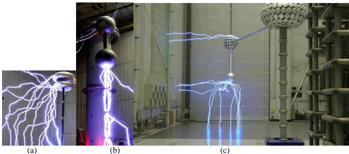
Figure 4. Competitive gaps during UHV testing. (a) Breakdowns from shielding of equipment HV shield. (b) rain test – notice streamers and breakdowns from top electrode and marx generator. (c) weak connection tube HV testing
