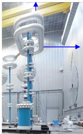
Figure 3. DC generator and damping resistors. Critical distances to walls, roof and ceiling marked.
