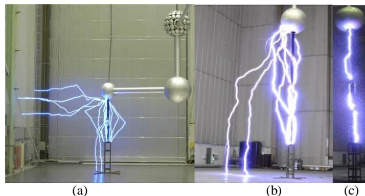
Figure 1. Photograph of UHV indoor test under switching impulses. From left to right: (a) 1.6 m diameter sphere with 10.6 m insulation, and (c) sphere of 2.0 m diameter with 8.5 m insulation under rain condition, all over pedestal of 2.4 m. Notice that the proximity effect of grounded planes is observed on the trajectory of the discharges.
