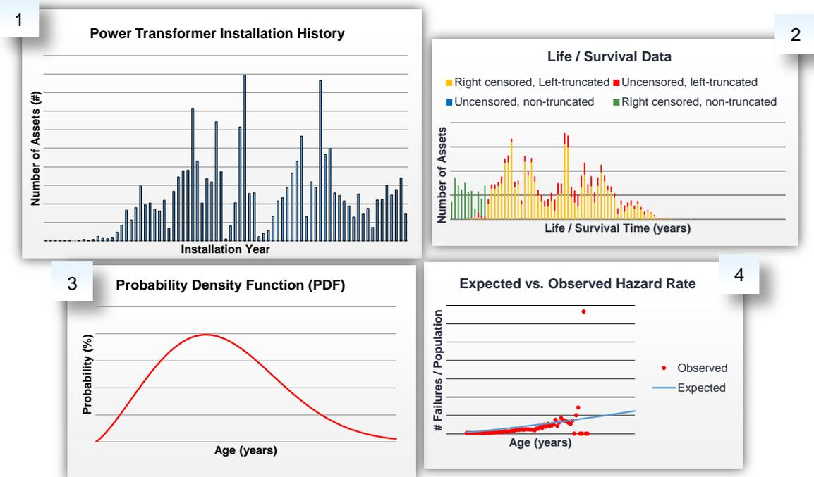
Figure 1 – Development of Age-Based Hazard Rate Function for Substation Assets
