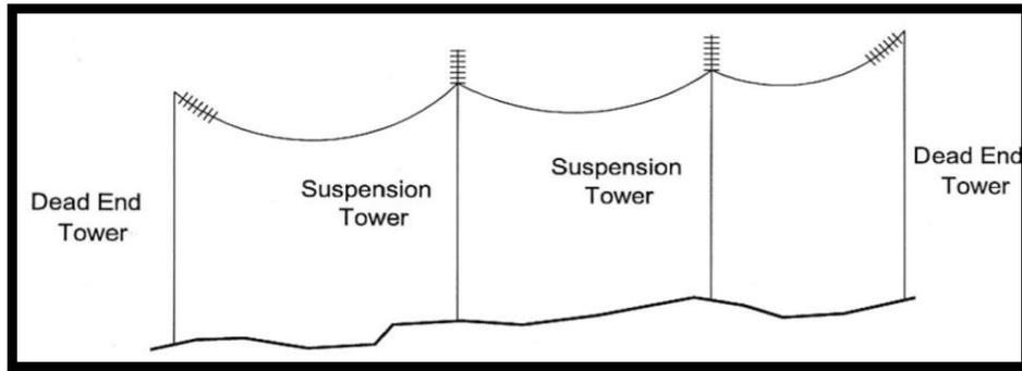
Figure 4 – Typical Line Layout
