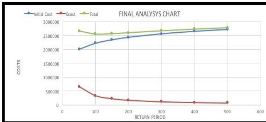
Figure 6– Optimum Return Period for a Lattice Steel Tower
