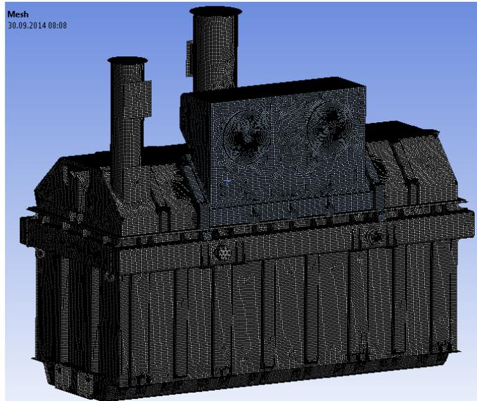
The support of the tank in the simulation is dependent in the physical positioning of the transformer or reactor unit during operation. Such constraints that may be simulated include: welded foundations; bolts; and units standing on wheels. An elastic support may also be employed to simulate an installation on rubber.
