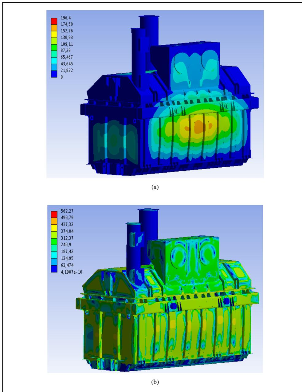
FIG. 5 (A) EXAMPLE OF THE STRAIN ON A TRANSFORMER TANK COMPRISING OF MILD STEEL AND STAINLESS STEEL PARTS AND (B) DETAIL OF STRAIN ON THE TANK
