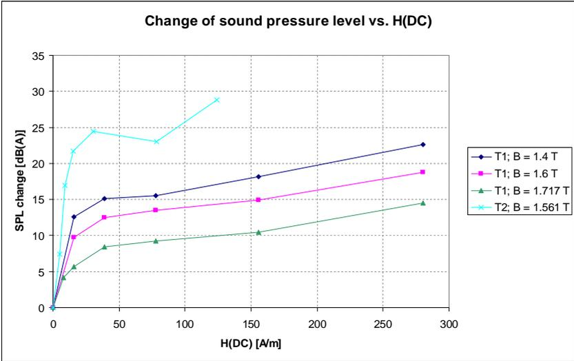
FIG. 2 CHANGE OF SOUND PRESSURE LEVEL AS A FUNCTION DC MAGNETIZATION.
