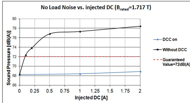
FIG 8. SOUND PRESSURE AT RATED INDUCTANCE AND DIFFERENT DC LEVELS FOR TRANSFORMER 1.
