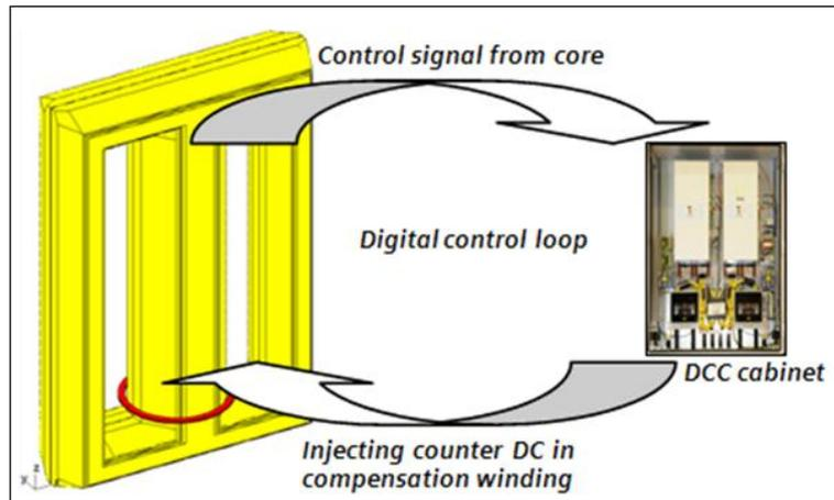
FIG 6. PRINCIPLE CONCEPT OF THE DC COMPENSATION.
