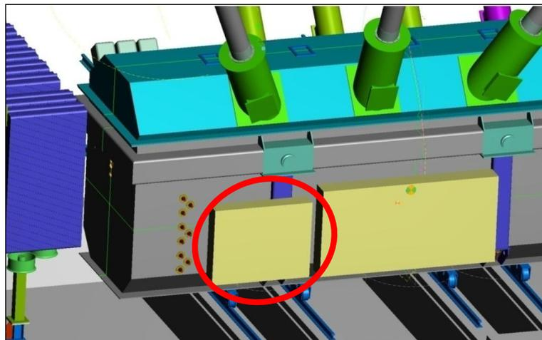
FIG 7. DC COMPENSATION CABINET (MARKED WITH RED CIRCLE) MOUNTED ON THE TANK.
