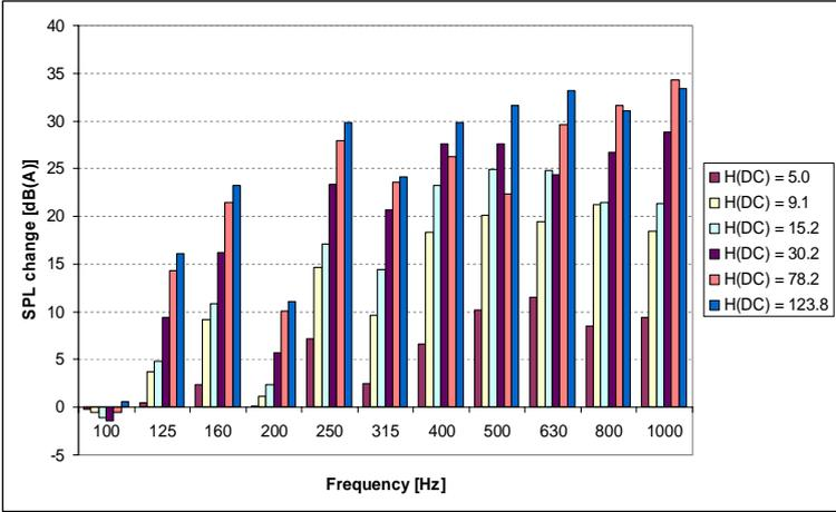
FIG 3. CHANGE OF SOUND PRESSURE LEVEL RESULTING FROM DC MAGNETIZATION (THIRD OCTAVE BANDS OF NO-LOAD NOISE OF TRANSFORMER 2).
