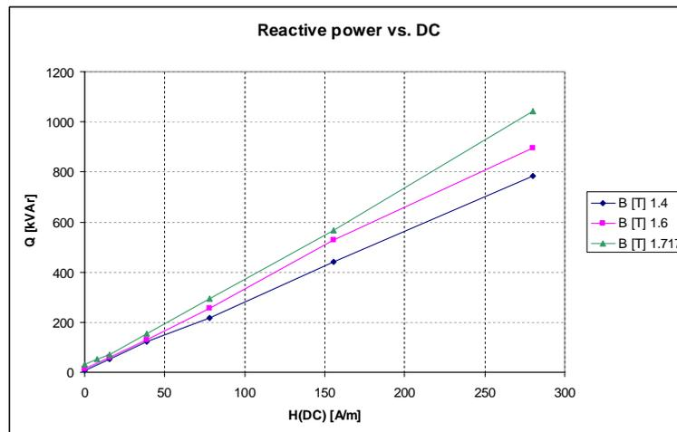
FIG 5. REACTIVE POWER CONSUMPTION AS A FUNCTION OF DC MAGNETIZATION AT DIFFERENT INDUCTION LEVELS FOR TRANSFORMER 1.
