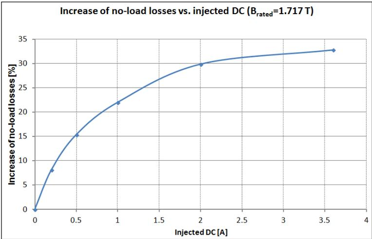
FIG 4. INCREASE IN THE NO-LOAD LOSSES OF TRANSFORMER 1 UNDER DC BIAS.
