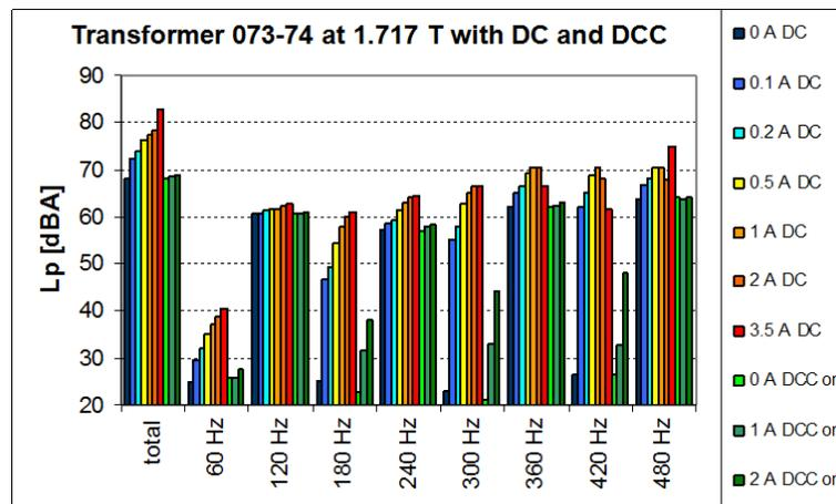
FIG 9. SPECTRUM OF SOUND PRESSURE LEVEL WITH DIFFERENT LEVELS OF DC AND DC COMPENSATION.
