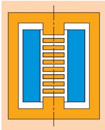
Fig. 3 Single-phase gapped core with return limbs [2]
