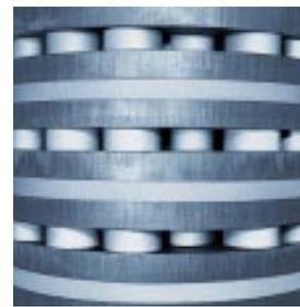
Fig. 1 Radially stacked core packages with ceramic spacers [2]
