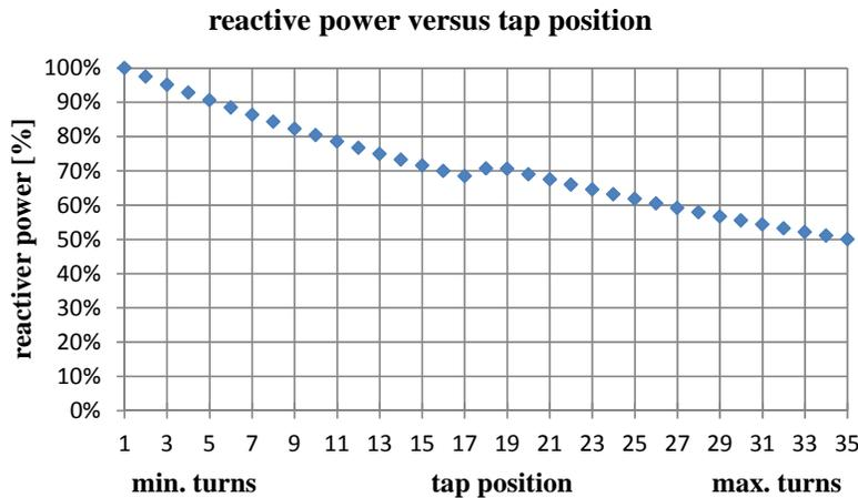
Fig. 4 Reactive power steps and regulation range of the VSR
