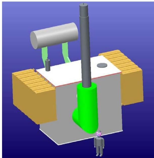
Fig. 6 Variable shunt reactor design
