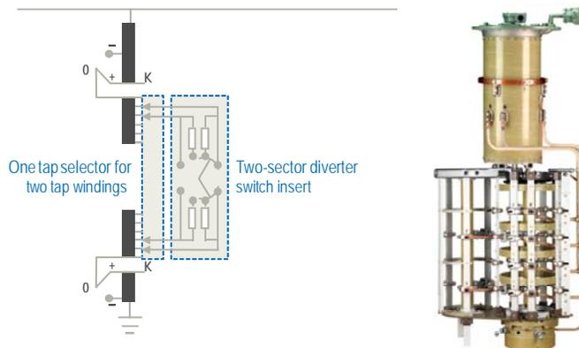
Fig. 2 Advanced OLTC design with two diverter switch sectors and optimized tap selector
