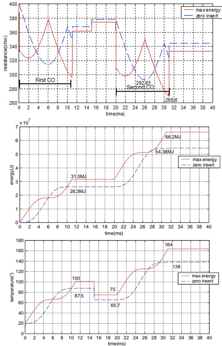
Figure 3 Resistor disc thermal and temperature simulation result
