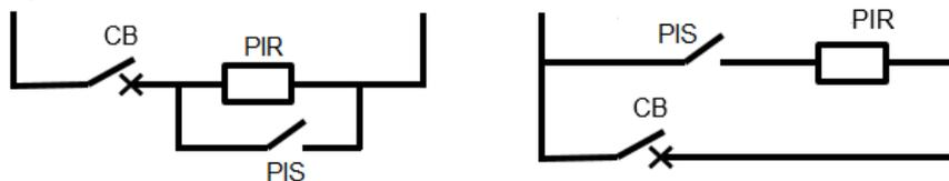
Figure 1 Resistor connected to CB in series (left) and in parallel (right)
