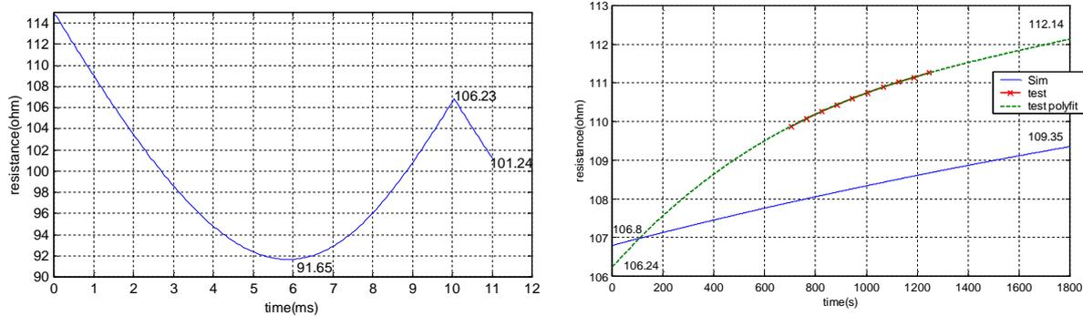
(a) Resistance during first CO; (b) Simulated (blue line) or measured (red cross) resistance
