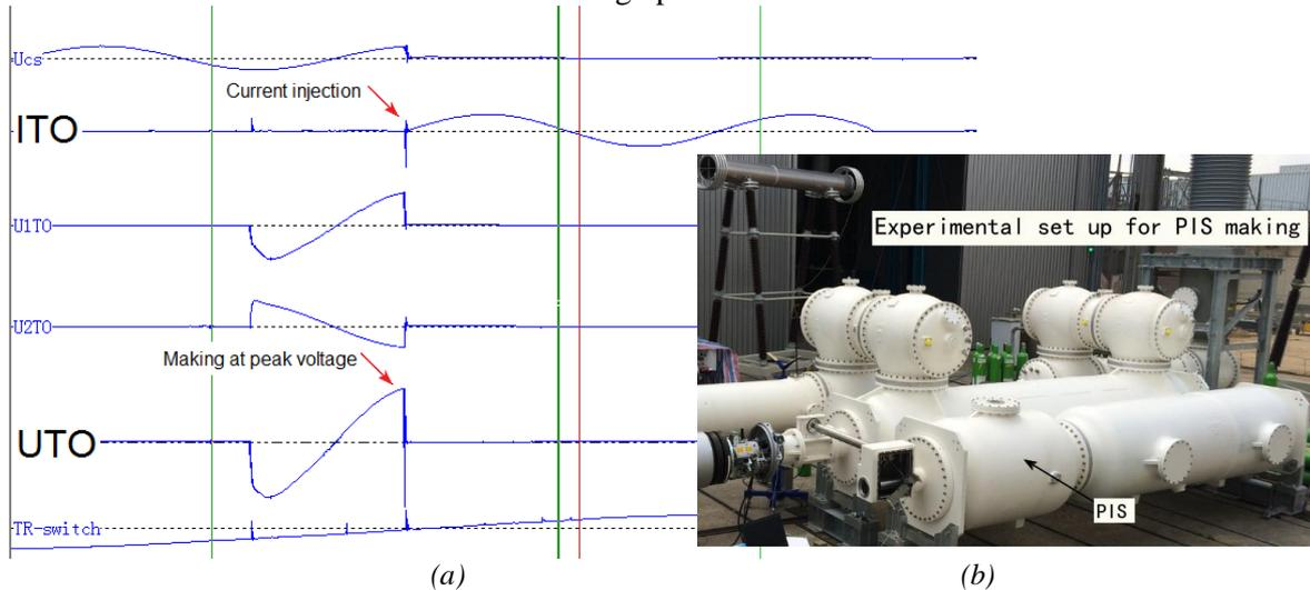
Figure 5 (a) one typical PIS making test and (b) test object for making test
