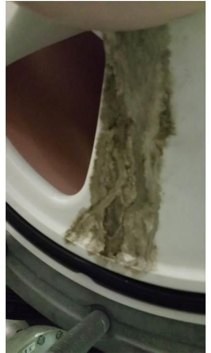
**Right – failure on insulator during site High Voltage test**
