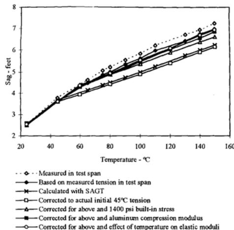
**Figure 3: Measured and Predicted Sag Values from EPRI Tests [10]**
