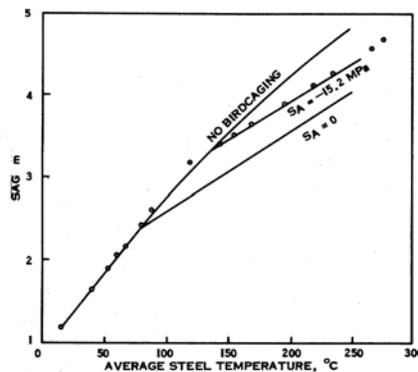
**Figure 2: Measured Sag in a 122 m outdoor test span [9]**
