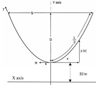
**Figure 1: Catenary Curve of a Level Span [2]**
