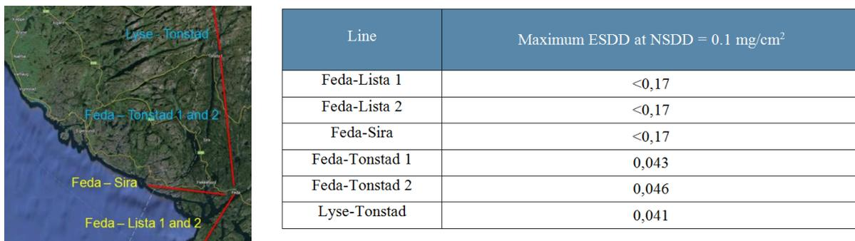
Figure 4 Left: Existing 300 kV AC lines in the area of interest; Right: ESDD levels for AC lines calculated using IST program.
