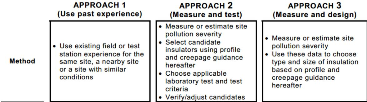
Figure 1 Three basic approaches to insulator selection and dimensioning (adopted from [4]).
