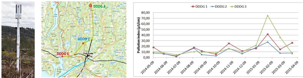
Figure 5 Left: Example of installed DDDG; Middle: Location of three DDDGs along the future route of NordLink; Right: Monthly measurements of DDDG Pollution index (1 year period).
