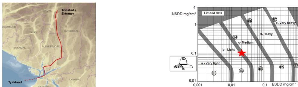
Figure 3 Left: Route of the NordLink line; Right: Relationship between ESDD and NSDD and environments E1-E7. The margin E2/E3 environment is marked by a red star.
