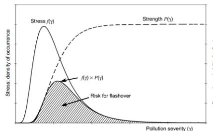
Figure 2 Principles of statistical dimensioning according to Annex G of IEC 60815-1 [4].
