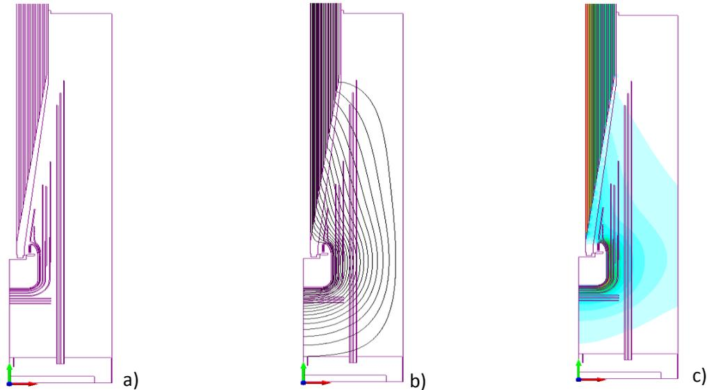
Figure 2 The AC field modeling of the 500kV DC bushing test system under  $850 \text{ kV}_{RMS}$ : a) geometry, b) equipotential lines, c) electric field distribution
