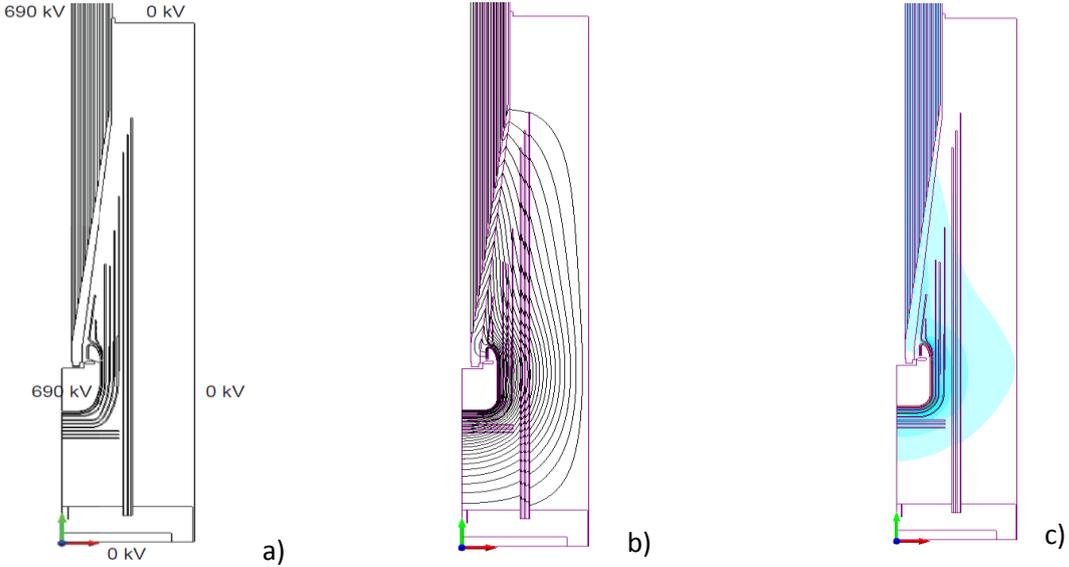
Figure 4 The PR field modeling of the 500kV DC bushing test system using DC-2-AC method under 690 kV: a) geometry, b) equipotential lines, c) electric field distribution
