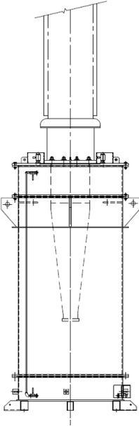
Figure 1 Example of a test tank – for 500kV DC bushing testing (moulded pressboard insulating system not shown)
