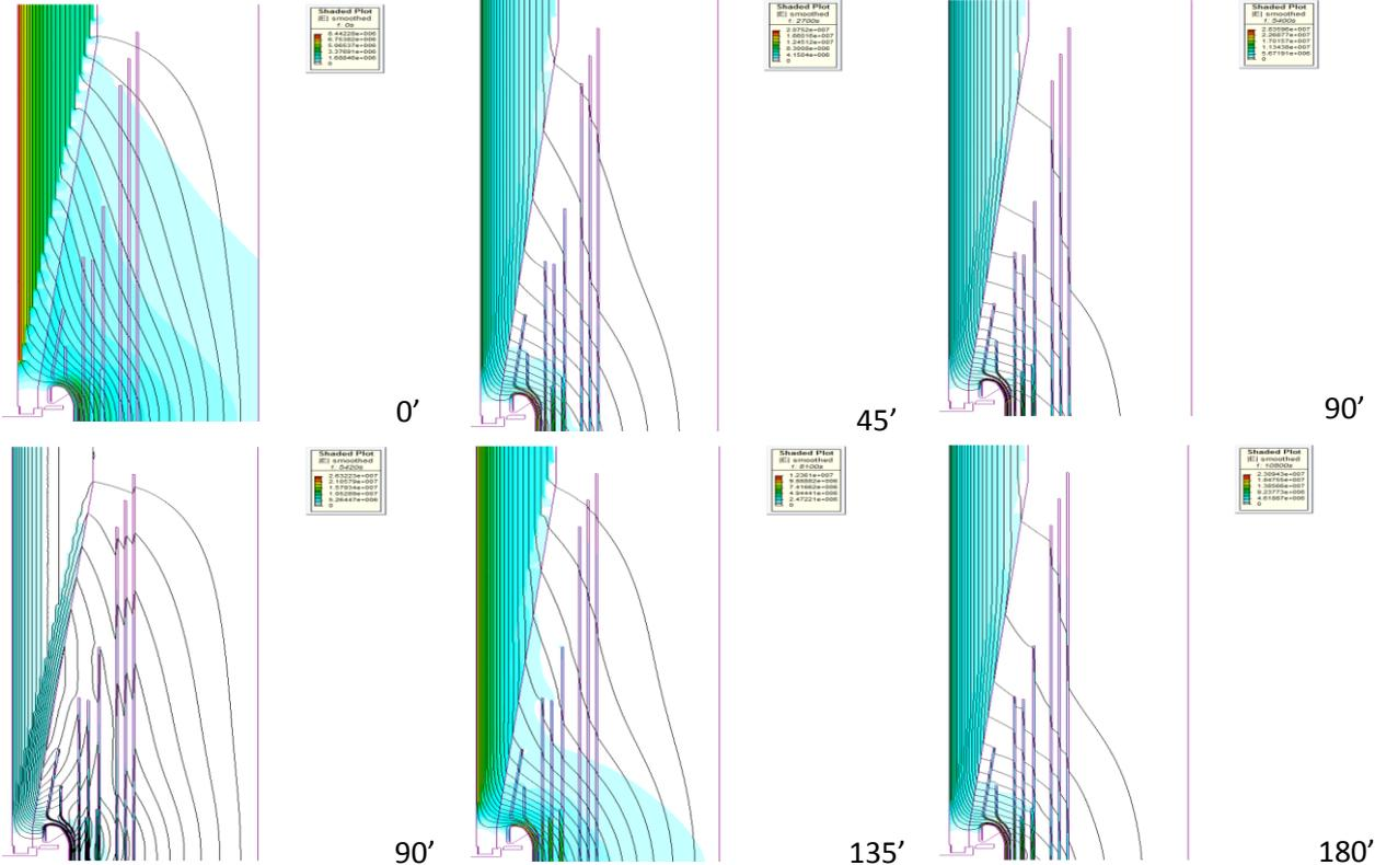
Figure 5 The electric field distributions during polarity reversal test as a function of time [minutes]: -690kV for first 90 minutes, +690 kV for next 90 minutes (remaining final 45 minutes at -690 kV not shown);
