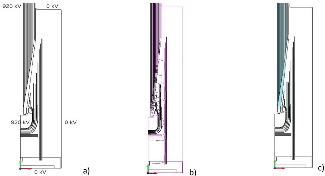
Figure 3 The DC field modeling of the 500kV DC bushing test system under  $920 \text{ kV}_{DC}$ : a) geometry, b) equipotential lines, c) electric field distribution
