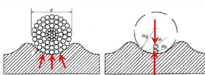
The benefit of the harder material applied for years to traditional conductors became more evident when HTLS conductors have been introduced into the market.
