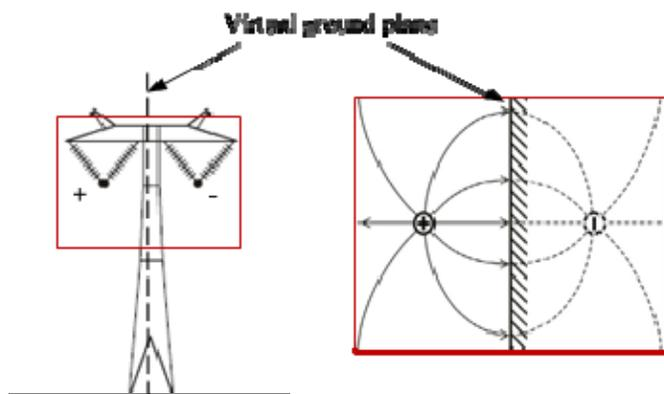
**Figure 1 : Virtual Ground Plane Representation of Bipolar DC Line**
