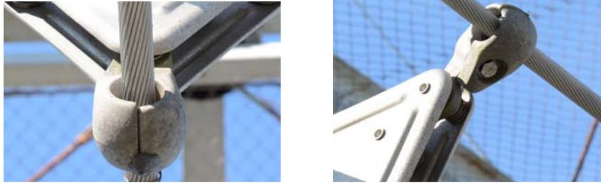
**Figure 5: Spacer damper in outdoor cage with a conic source (left) and with a spherical source (right)**
