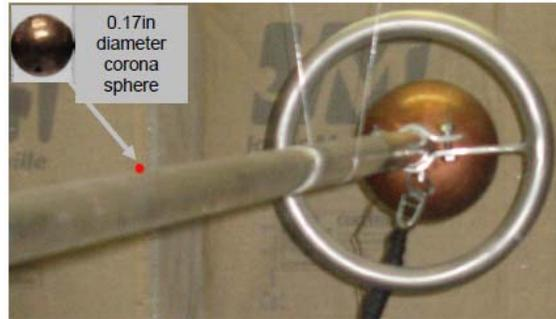
**Figure 2: Corona Calibrating Sphere in Corona Cage**
