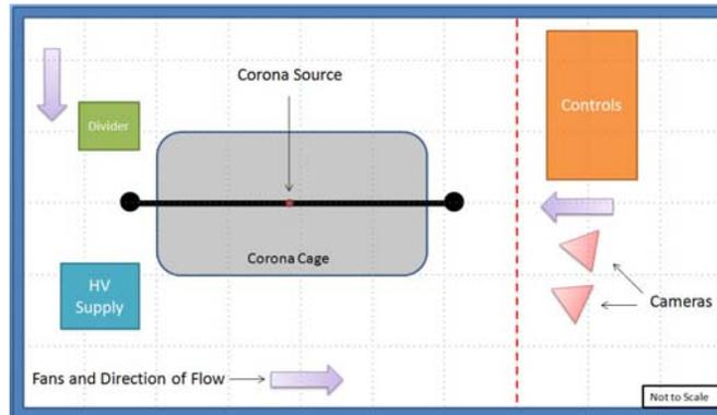
**Figure 3 : Diagram of Test Setup**
