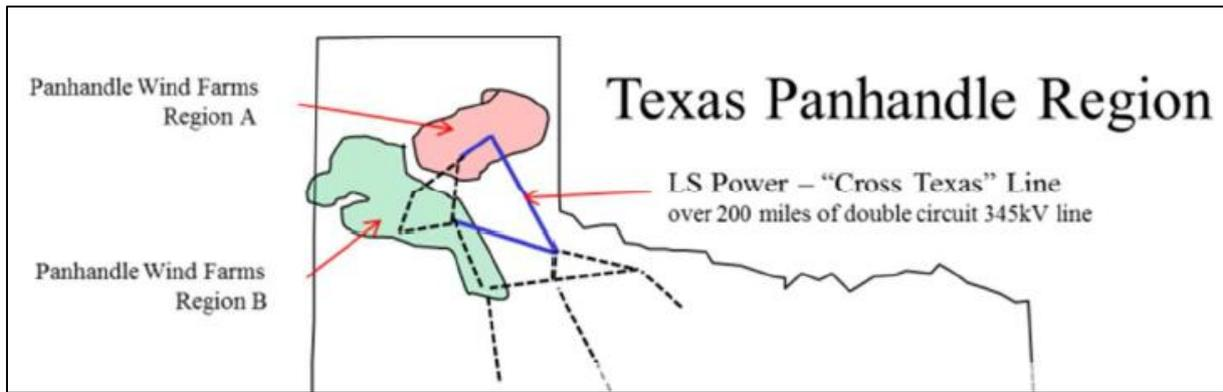
Figure 4 - Layout of new 345 kV Double Circuit Line
