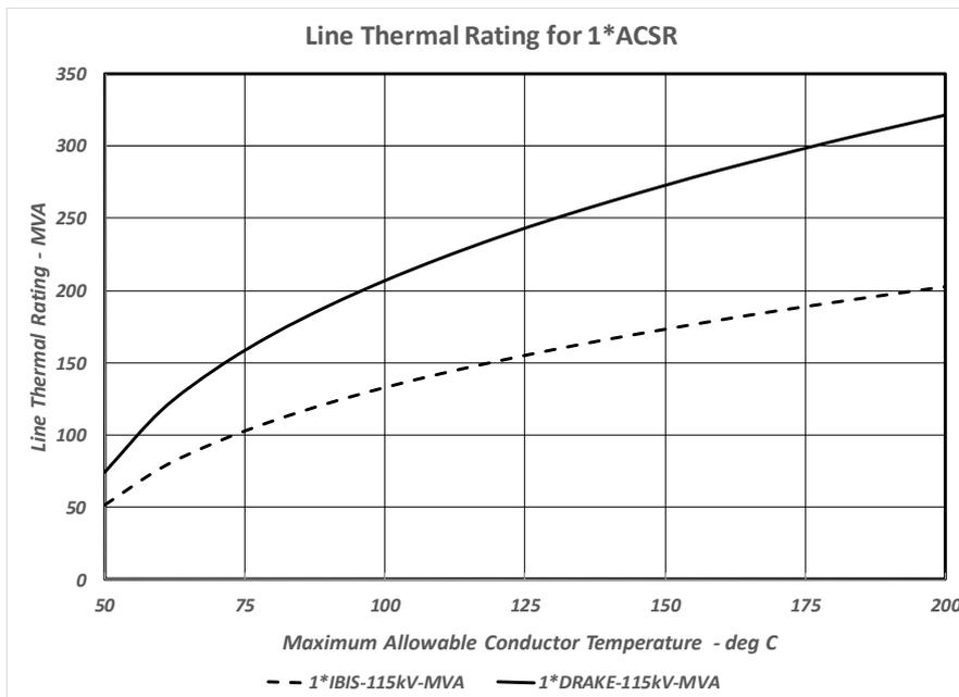
Figure 2- 115 kV Line Thermal Rating vs MACT for Single Ibis (397.5 kcmil) and Drake(795kcmil)
