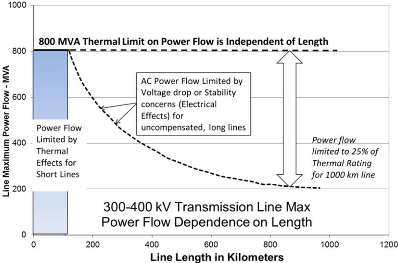
Figure 3 - Power Flow Capacity Limits versus Line-Length
