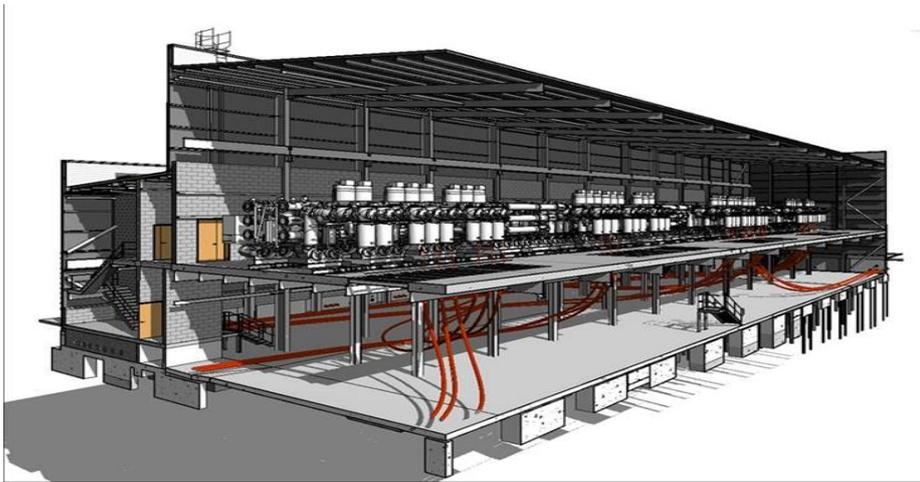
**Figure 5: 3D Model View of 400 kV Building and Switchgear**
