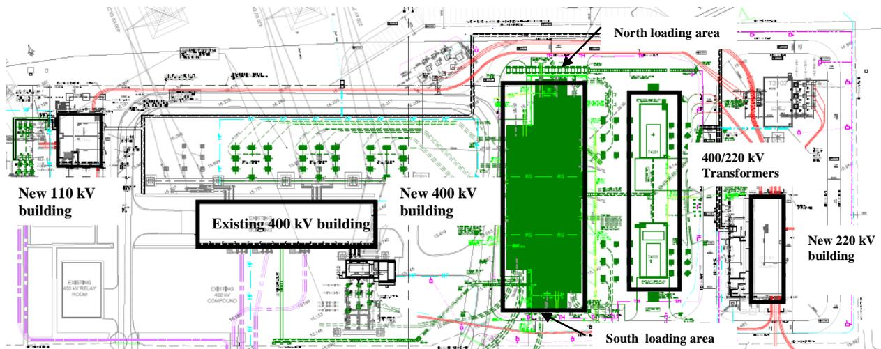
**Figure 3: Overview of Moneypoint 400 kV substation and underground services**
